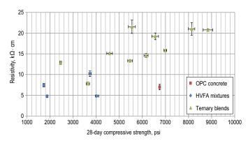
Fig. 9: Surface resistivity (56 day) as a function of 28-day compressive strength for the 15 concrete mixtures. Error bars indicate  $\pm$  one standard deviation for the measured data (Note: 1000 psi = 6.9 MPa)
