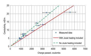
Fig. 8: Calculated specimen conductivity as compared with cumulative charge passed for the 15 concrete mixtures. Diagonal lines indicate model relationships for calculations that are performed with and without the effects of Joule heating of the specimens being included.<sup>21</sup> Error bars indicate ± one standard deviation in measured charge passed
