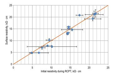
Fig. 6: Measured surface resistivity as compared with resistivity calculated from initial current in the RCPT (both at 56 days) for the 15 concrete mixtures. The diagonal line indicates the expected one-to-one relationship. Error bars indicate  $\pm$  one standard deviation for the measured data
