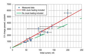
Fig. 5: Measured cumulative charge passed over 6 hours (RCPT) as compared with measured initial current (both at 56 days) for the 15 concrete mixtures. Lines indicate conversion of initial current to cumulative charge passed with (current changes with temperature) and without (constant current) a Joule heating correction.<sup>18</sup> Error bars indicate ± one standard deviation for the measured data
