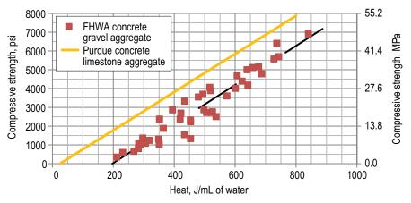
Fig. 1: Measured compressive strength as a function of measured cumulative heat release (per unit volume of water). The strength-heat release relationship (dashed line) is a best-fit line used for adjusting mixture proportions. The relationship labeled as Purdue concrete is based on data from Reference 14
