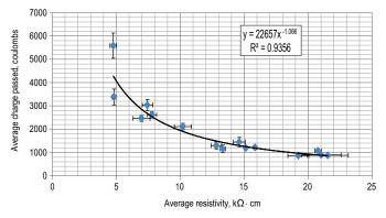
Fig. 7: Average cumulative charge passed (RCPT) as a function of measured average surface resistivity at 56 days for the 15 concrete mixtures. Error bars indicate  $\pm$  one standard deviation for the measured data
