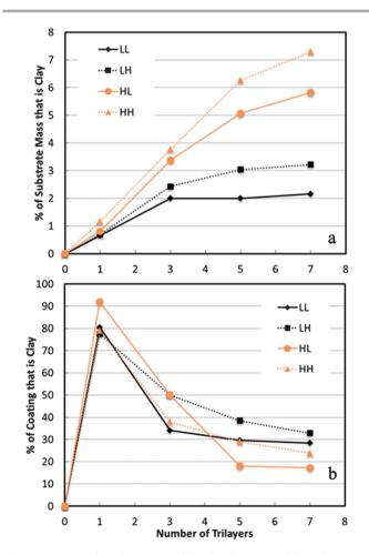
**Fig. 7** MMT mass% on the substrate (a) and in the coating (b) as a function of the number of TLs deposited on the foam.
