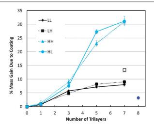
Fig. 2 Mass growth of LL, LH, HH and HL systems of PU foam as a function of TL numbers. 8 TLs from a previous study ((0),<sup>31</sup> and LH 7 with the dipping solutions refreshed at 4 TLs ( $\Box$ ) are also shown for comparison.
