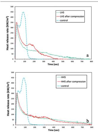
Fig. 9 Heat release rate of LH3 (a) and HH5 (b) foam after the compression and aging.
