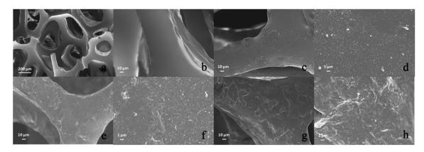
Fig. 3 SEM images of control foam (a and b), LH1 (c and d), LH3 (e and f), and HH7 (g and h) coated foams.
