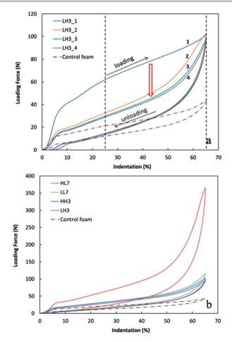
**Fig. 8** Loading–displacement curves for (a) uncoated PUF (first compression cycle) and LH3 as a function of the number of compression cycles and (b) for the best flammability reduction with the least number of TLs for each formulation (fourth compression cycle).
