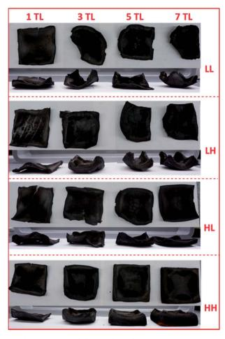
Fig. 5 The photographs of all coated foam after cone calorimetry.
