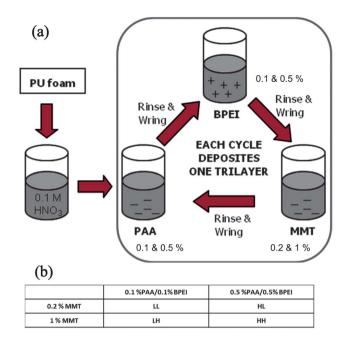
**Fig. 1** (a) Schematic of the LbL deposition process on PU foam. Foam was first dipped in an acidic solution and placed in coating solutions without rinsing. The foam was coated with PAA, BPEI and then MMT, until the desired number of layers was reached. Between each deposition the foam was rinsed with DI water. The concentrations of the dipping solutions are listed, and the concentrations of the solutions for four different systems: LL, LH, HL, and HH are listed in (b).
