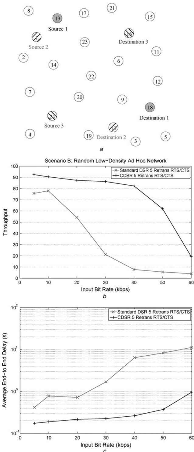
**Fig. 10** Scenario B: a multi-session scenario in a low-density wireless sensor network. The proposed CDSR scheme is capable of achieving partial cooperative diversity and improving the performance
