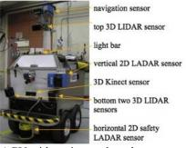
Figure 6a. AGV with various onboard sensors.
