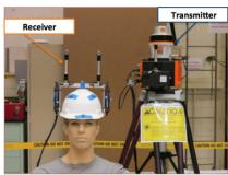
Figure 3. iGPS vector bar attached to hardhat worn by a human (represented here by a mannequin).
