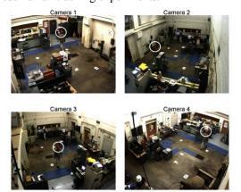
Figure 7: Different camera views during a test. Note the hardhat being tracked by the iGPS system (white circle). [14]
