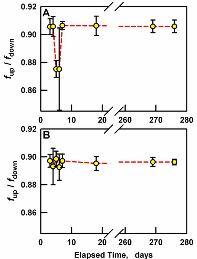
Figure 4. The ratio of the upstream rotor frequency to the downstream rotor frequency during 8 calibrations spanning almost a year. A) Turbine meter that was rinsed and dried in between each calibration. B) Turbine meter that was left continuously in reverse osmosis water. The error bars shown are the standard deviation of 7 measurements.
