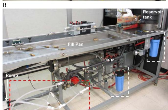
Figure 2. A) The 2.5 L/s LFS. B) The 0.1 L/s LFS. The plumbing that was replaced is outlined in red. The filters that were added are outlined in white.
