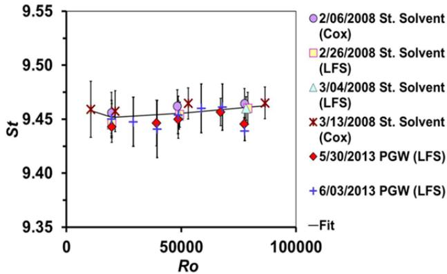
Figure 6. Validation of the calibration of a 1.25 cm PD meter in Stoddard solvent and 5 % PG + W mixture. The error bars shown are the RSS of the LFS uncertainty and the standard deviation of the PD meter measurement at a confidence level of approximately 95 %.
