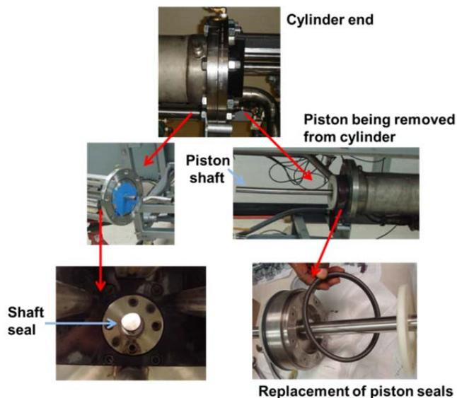
Figure 3. The cylinder of the 2.5 L/s LFS disassembled for cleaning and seal replacement.
