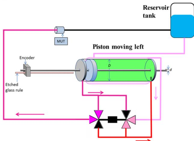
Figure 1. Sketch of the piston prover with the piston stroking left.
