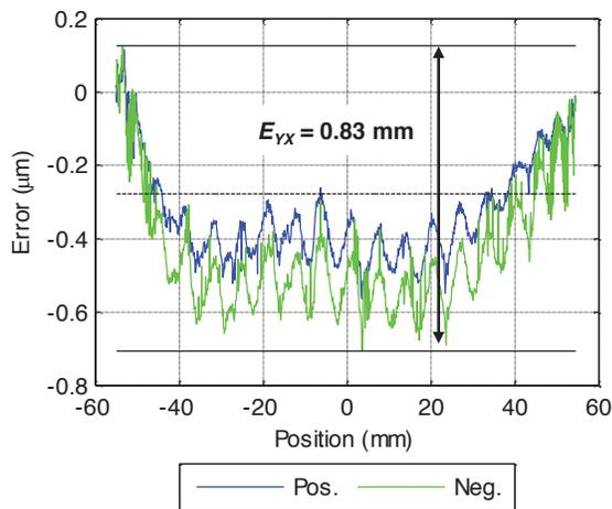
**FIGURE 5.** Illustration of a unidirectional dynamic straightness plot.
