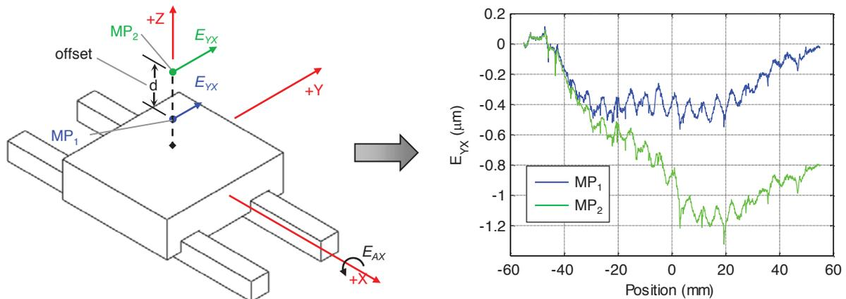
FIGURE 2. Straightness errors of a linear positioning system at two measured points (MP).
