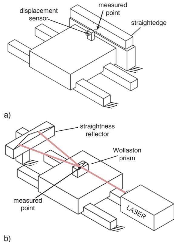
*FIGURE 3. A schematic illustrating moving sensor measurement setups; a) displacement sensor measuring against a straightedge artifact b) straightness interferometer using a Wollaston prism.*
