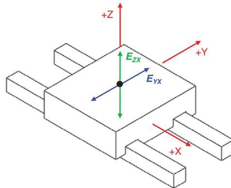
FIGURE 1. A schematic identifying the straightness errors of a linear positioning system traversing in the x-direction.  $E_{yx}$  and  $E_{zx}$  represent the straightness error motions in the y- and z-directions, respectively.
