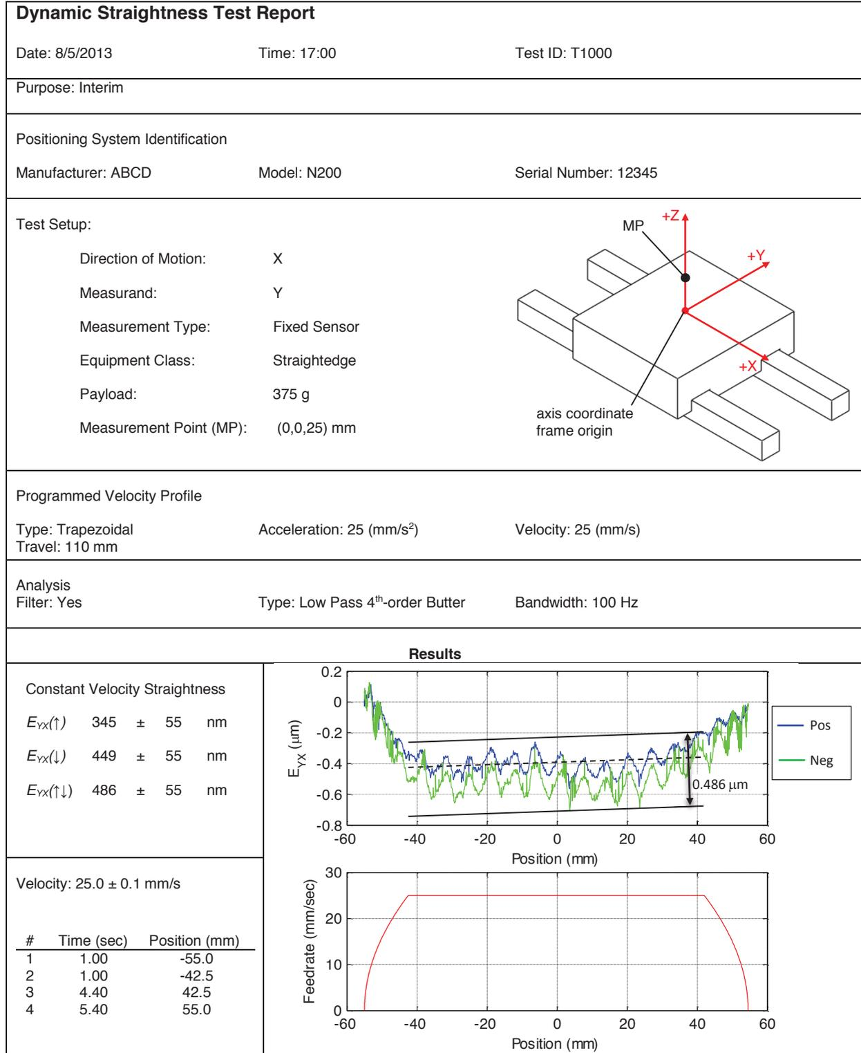
FIGURE 6. Example of a dynamic straightness report.
