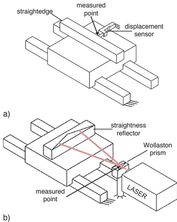
FIGURE 4. A schematic illustrating fixed sensitive measurement setups; a) displacement sensor measuring against a straightedge artifact b) straightness interferometer using a Wollaston prism.
