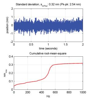
FIGURE 3. Example In-position jitter measurement results for a direct-drive, linear positioning axis.
