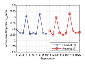
Figure 5. Incremental step sizes,  $X_{inc}$ , calculated from the 2.5 nm commanded incremental step test example.
