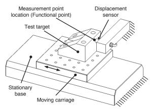
FIGURE 1. Example measurement setup for a linear axis step test showing the measurement of displacement at the functional point.
