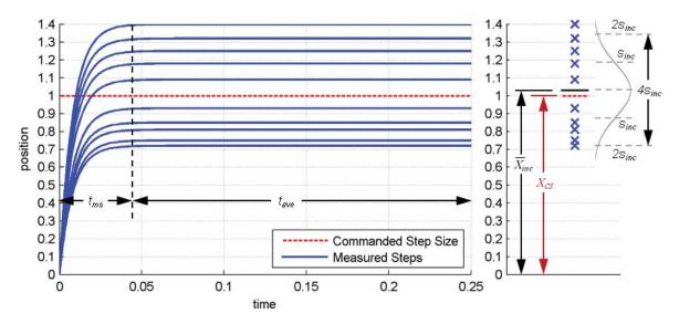
Figure 6. Illustration of Criterion A2 and A3 for determining if a positioning axis passes or fails an Incremental Step test.
