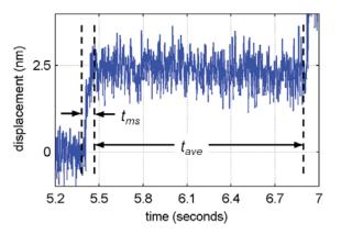
Figure 4. Illustration of the move-and-settle time,  $t_{ms}$ , and the average time,  $t_{ave}$ .
