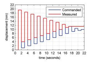
Figure 7. Successively alternating, decreasing steps used to measure the Incremental Step Reversal Error.
