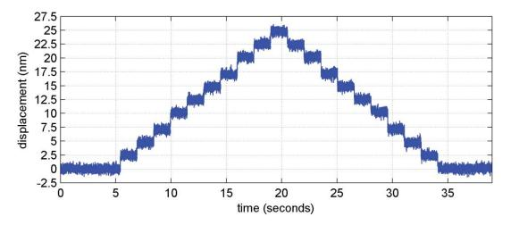
Figure 2. Example time verses displacement plot for an Incremental Step Test performed on a direct-drive linear positioning axis with a 2.5 nm commanded step size.
