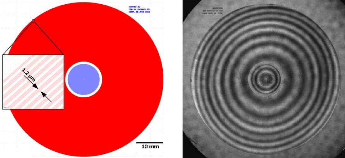
Figure 2. Layout of the nested zone lens (left) and interferogram obtained with the measurement setup shown in Fig. 1 (right). The inner zone lens has a diameter of 12 mm, the outer zone lens a diameter of 60 mm.
