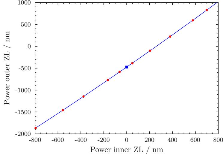
Figure 4. Measured power in the outer zone lens as function of the power in the inner zone lens (red data points) and a quadratic fit to the data (blue line). The power in the outer zone lens area at zero power in the inner zone lens area is -474.22 nm.
