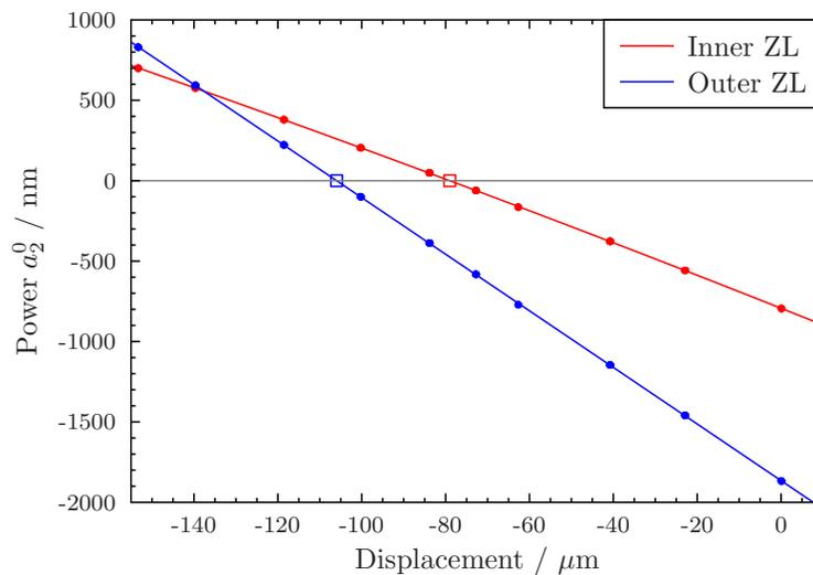
Figure 3. Defocus in the inner (blue) and outer (red) zone lenses as a function of displacement. A positive displacement moves the test sphere towards the nested zone lens. The curves are least-squares best-fit quadratic polynomials calculated from the measurement data.
