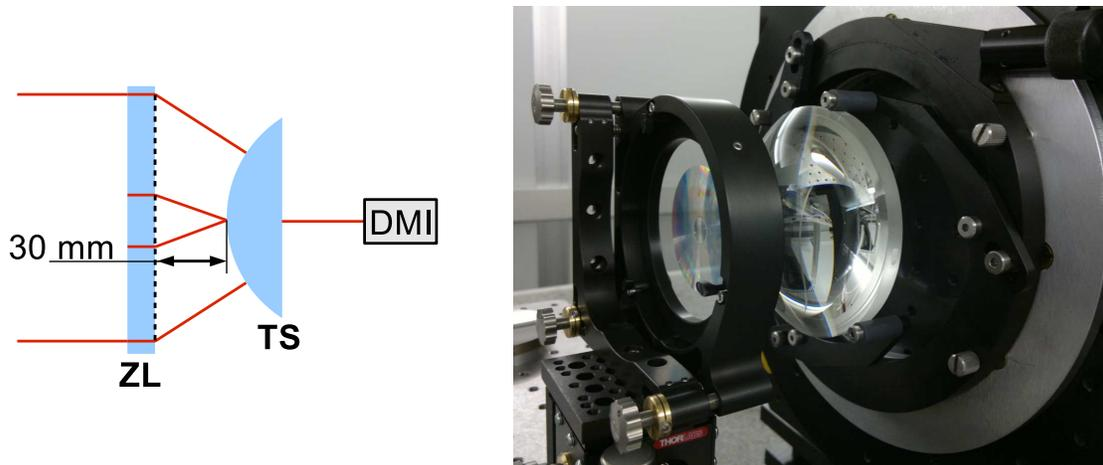
Figure 1. Setup for the radius measurement of a precise test sphere (TS) with 80 mm radius using a nested zone lens (ZL). A displacement-measuring laser interferometer (DMI) tracked the movement of the test part along the optical axis. A sketch of the setup is shown on the left, a photograph of the actual setup on the right.
