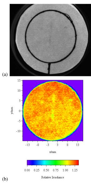
**Figure 7.** Example of the irradiance uniformity at 253.7 nm. A photograph (a) from the camera mounted above the water sample imaging the fluorescence from typical card stock paper. The dark circle marks the area of the water sample Petri dish. A plot (b) of the relative irradiance uniformity normalized to the beam center.
