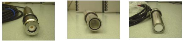
Figure 1. Photos of example UV sensors used in water disinfection.
