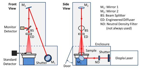
**Figure 4**. The NIST tunable UV irradiance laser system optical configuration. The Standard Detector is substituted for the Sample to measure the irradiance at each wavelength of interest.
