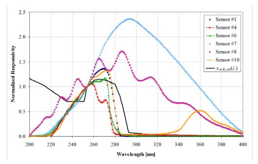
**Figure 2.** Plot of the relative spectral responsivities of six of the UV sensors measured. Also shown is the microbicidal action spectrum,  $s_{\text{mik,rel}}(\lambda)$ .
