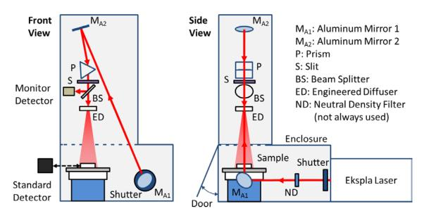
**Figure 5.** The NIST tunable UV irradiance laser system optical configuration for 210 nm to 230 nm. The dielectric mirrors are replaced by aluminum mirrors and a prism and slit are added.
