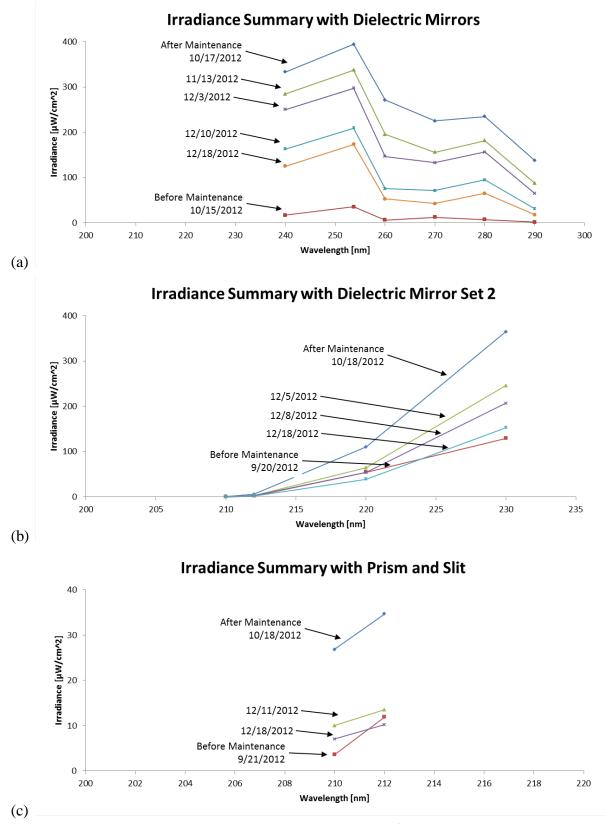
**Figure 8.** Graphs showing the decrease in irradiance  $(\mu W/cm^2)$  over time and the improvement when some of the damaged EKSPLA laser optical components were replaced.
