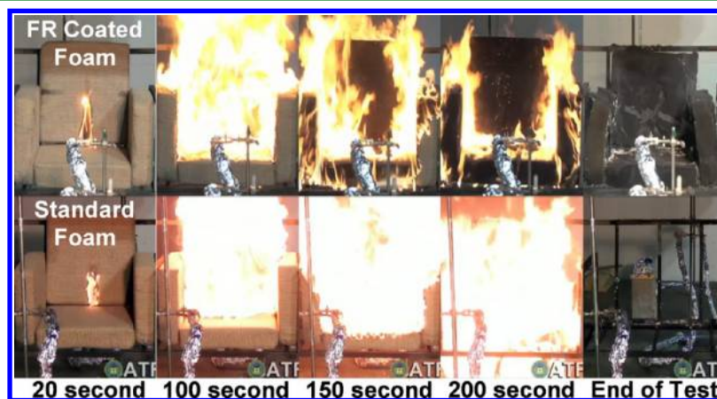
Figure 5. Images captured from the real scale fire test (captured from video records). The test is completed by approximately 250 s for the control PUF, which is completely consumed at the end of the test. The FR coated sample test lasts for 400 s, and it is still partially intact and maintains its shape.
