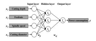
Fig. 6. A structure of neural network.
