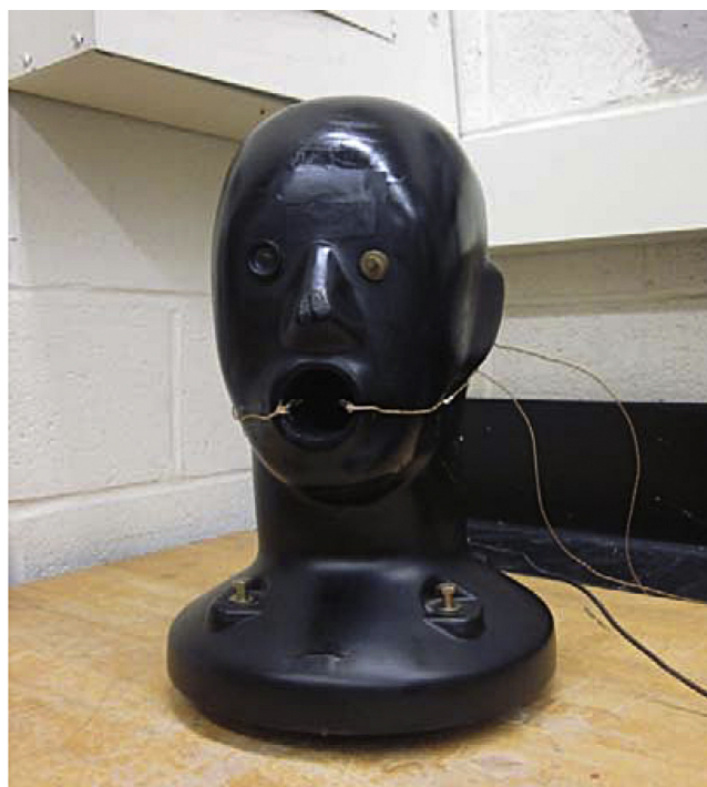
Fig. 3 – Mannequin headform with thermocouples inside mouth.
