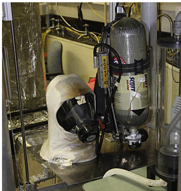
Fig. 2 – SCBA equipment on the flow loop testing platform.
