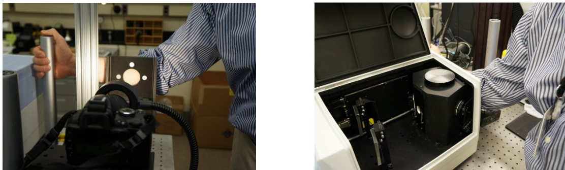
Figure 1. On the left, the imaging setup showing the exposed sample area of the skin. The white and grey scale references surround the aperture of the mask. The camera is positioned to view through the ring illuminator. On the right, the spectrophotometer is shown with the cover in the open position to illustrate the location of the integrating sphere in relation the arm.
