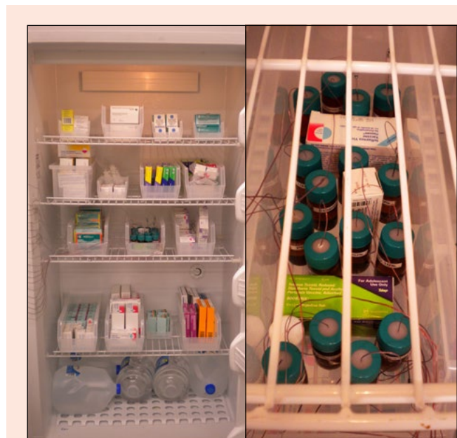
Figure 2. Figure 2a (left) shows refrigerator setup, with a test tray placed in the center of the refrigerator. Other trays are filled with vaccine boxes to produce a moderate-density load. Figure 2b (right) shows the 20 mL, varying buffer concentration setup tested in trials 1 and 2.
