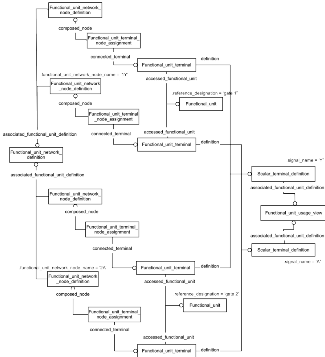
Figure 4. A Functional_unit_network_definition composed of two instances of a common functional element.
