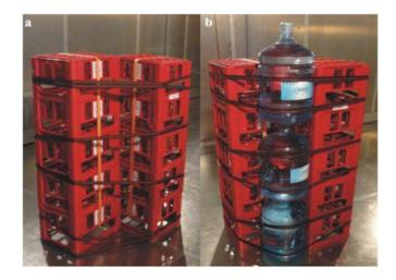
Fig. 5. Reverberation chamber interior for the water jugs measurements: a) Support structure and b) Cylindrical water model with support.
