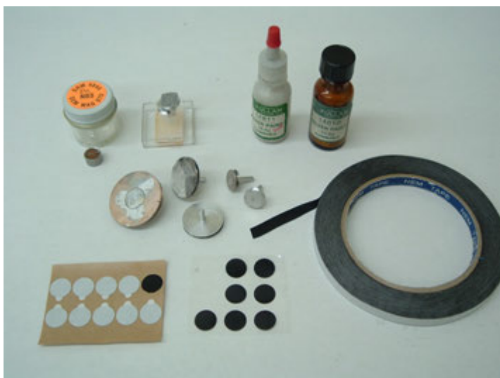
Figure 3.39 SEM specimen preparation tools. Clockwise from the top left are two SEM length calibration standards, two silver paint bottles, a double-sided conductive adhesive tape roll, two sheets of double-sided conductive adhesive disks, and an assortment of aluminum stubs.
