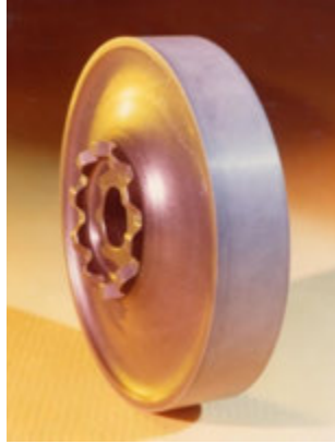
Figure 10.1. A Ford silicon nitride 95 mm diameter model gas turbine rotor that survived 25 h intact. The outer rim is thicker than a real rotor in order to simulate the mass of the vanes that would be attached in a real rotor.
