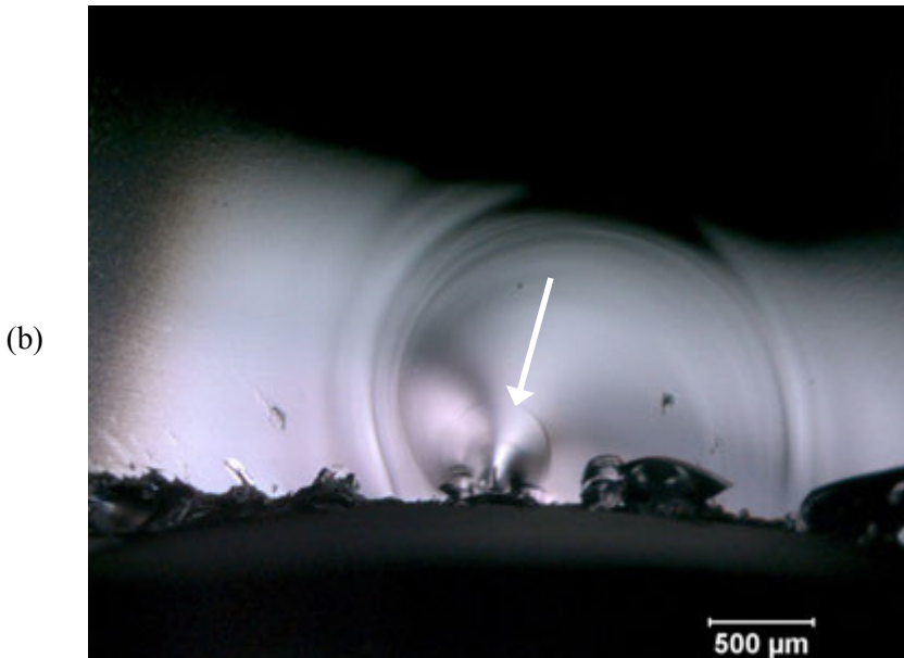
Figure 6.59 Very tiny chatter cracks from a small object that contacted and slid across the surface of a heat-strengthened soda lime glass kitchenware. (a) shows the outer surface with an assortment of common scratches and edge chips, some of which are secondary edge chips after the main fracture. The arrow points to the exact origin site which is seen to be one of a series of curved chatter cracks. (b) shows the fracture surface. The multiple secondary edge chips may confuse interpretation, but the Wallner lines and a faint pop in arrest line are centered on the chatter crack (arrow).
