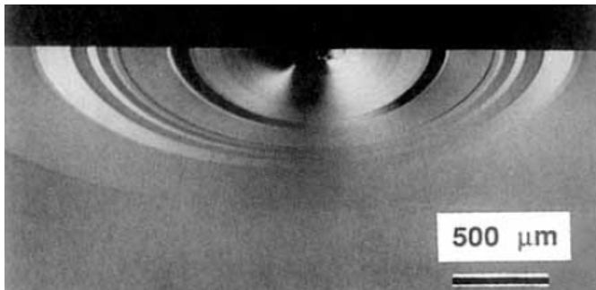
Figure 5.66 Concentric arrest lines in a plate of soda lime silica that was cyclically loaded in flexure. The lines are due to slight variations in the crack growth planes on each loading cycle. (courtesy of D. Green, Penn State University, same as Figure 5.47c)
