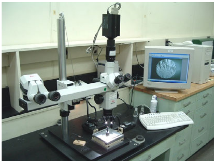
Figure 3.14 A discussion stereoptical microscope that allows two observers to simultaneously view an object. Note the very tall post (800 mm) on which the microscope body is mounted. The entire assembly can be moved up or down as required to facilitate examination of very large or very small specimens. Beam splitters in the optical path enable simultaneous viewing through the eyepieces at the same time the digital camera views the object.
