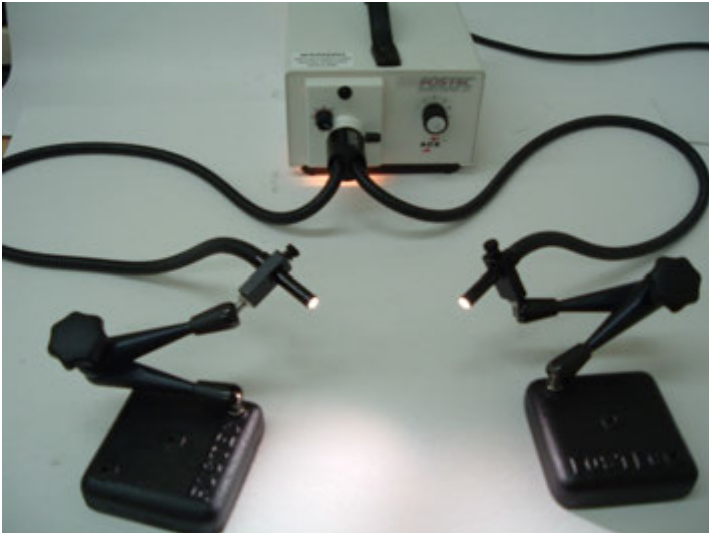
Figure 3.17 Dual gooseneck fiber optic light guides allow flexibility in directional illumination.
