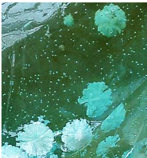
Figure 6.54 Unusually large ( \approx 1 cm) glass devitrification inclusions with a blossom-like structure as well as smaller seed bubbles. (Specimen courtesy of J. Varner and V. Fréchette)
