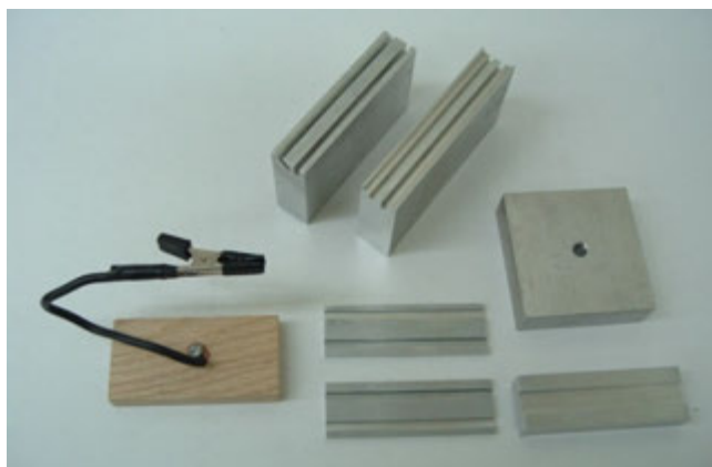
Figure 3.5 Specimen holders. Clockwise from the lower left are: a bend bar holder made with an alligator clip on a bendable (10 gage electrical) wire with electrical tape wrapped around the teeth to cushion the specimen, two aluminum jigs with slots and grooves for bend bars or tension strength specimens, an aluminum block with hole, and three aluminum holders comparable in size to a glass microscope slide with grooves to hold bend bars both on their flats and on edge for chamfer examination.
