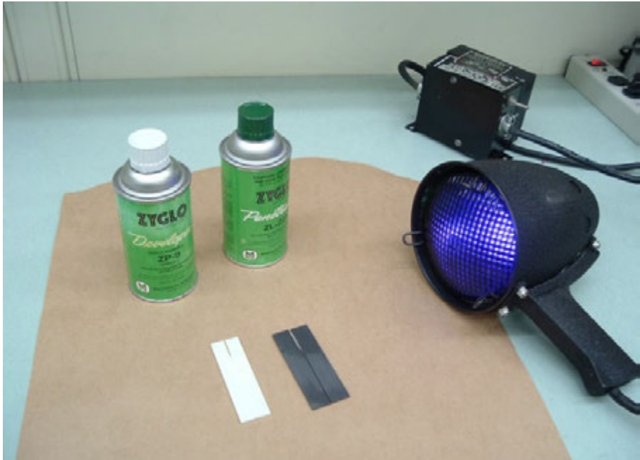
Figure 3.55 Fluorescent dye penetration equipment. Two double torsion specimens are shown. The white one is an alumina, the black one, a silicon nitride.
