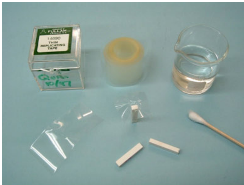
Figure 3.31 Thin cellulose acetate replica tape, acetone, applicator, and bend bar specimens. These are used to make reversed (negative) replicas.
