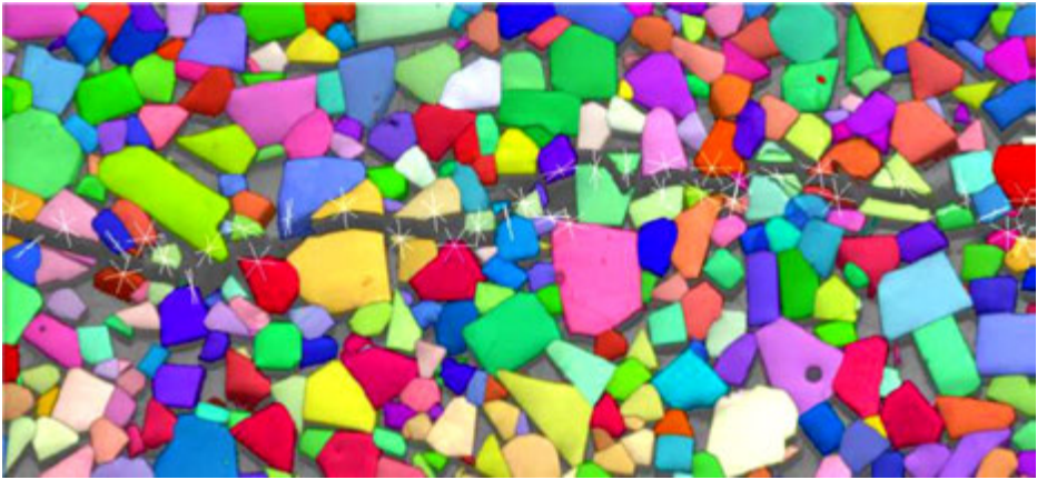
Figure 3.46 Electron backscatter diffraction map of the flat exterior surface of a tungsten carbide/11 mass % cobalt fracture toughness test specimen. The black crack has propagated through the microstructure. Individual grains with different crystallographic orientations are shown in color. Crack propagation was under static loading and was mixed inter- and transgranular, with the latter through the grains on [10\bar{1}0] slip planes. (Image courtesy of R. Morrell and K. Mingard, NPL)
