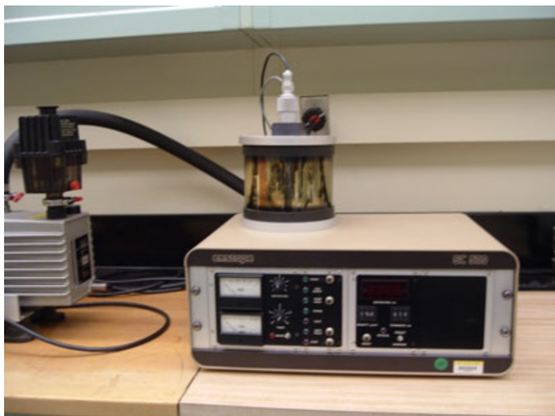
Figure 3.40 A gold sputter coater used to apply conductive coating. It is helpful for both optical and scanning electron microscopy.
