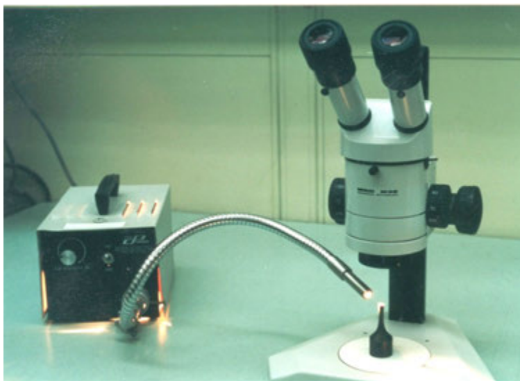
Figure 3.11 Stereo binocular microscope with a fiber optical light source for directional illumination. This is an indispensable tool for the ceramic and glass fractographer. “Low-angle, grazing illumination” is illustrated in the picture. In other cases, a ring light mounted on the objective lens of the microscope may be suitable. This particular microscope has interchangeable 0.63X, 1.0X and 2.0X objective lenses, a body zoom magnification range of .65X to 4X, and 25X eyepieces for an overall magnification range of 10X to 200X. The moderately tall (300 mm) mounting post enables specimens up to 150 mm tall to be placed under the microscope.
