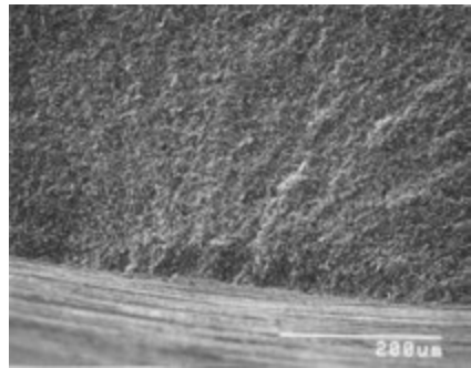
Figure 6.38 Examples of parallel grinding cracks. (a) and (b) show optical images of a “zipper crack” in a sintered silicon nitride bend bar. (d) and (e) show SEM images of a crack in a silicon nitride rod.
