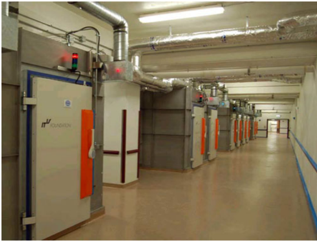
Fig. 5. RFR reverberation chambers installed at IITRI.
