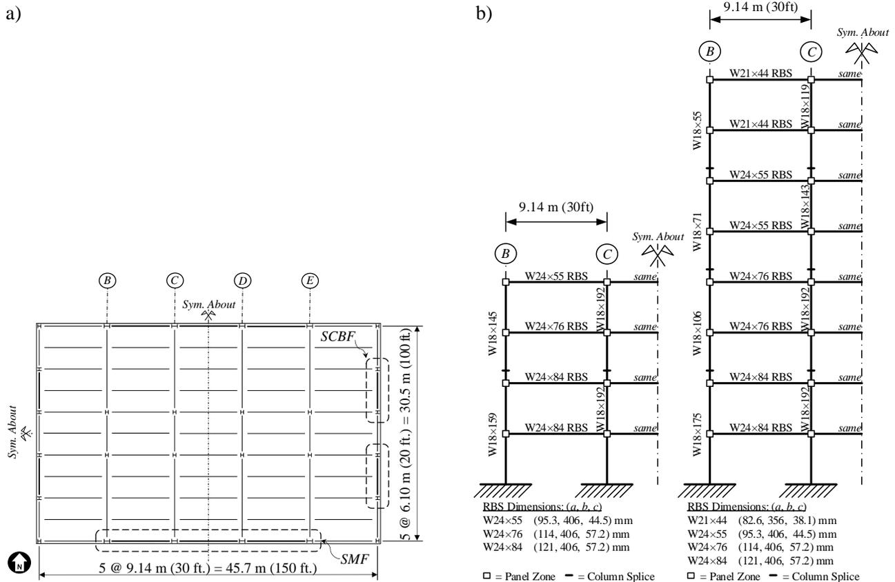
Fig. 2 – (a) Floor plan and (b) SMF elevations for the archetype buildings used in this study.
