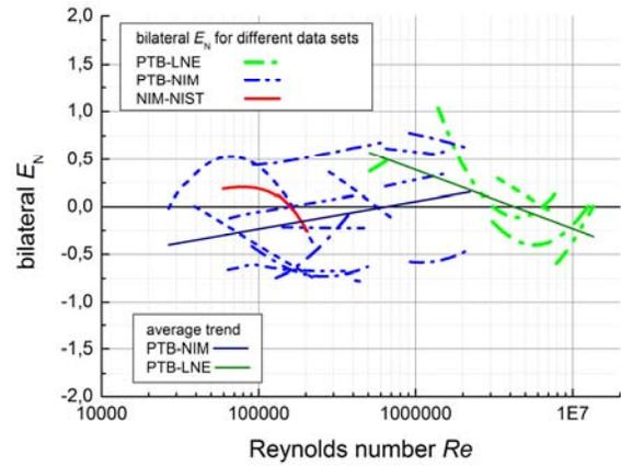
**Figure 4:** Bilateral  $E_N$  PTB-LNE, PTB-NIM and NIM-NIST for all nozzles and all datasets.
