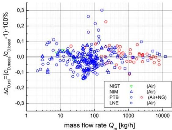
**Figure 5:** Differences  $\Delta c_D$  of single  $c_D$  values (relative in %) against the  $c_{D,base}$  functions for all nozzles and all measurement series.
