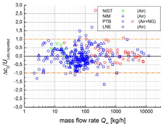
**Figure 6:** Normalised differences  $\Delta c_D / U_{Lab,reported}$  as shown in Figure 5 using the related uncertainties reported by the laboratories ( $k = 2$ ) for all nozzles and all measurement series.
