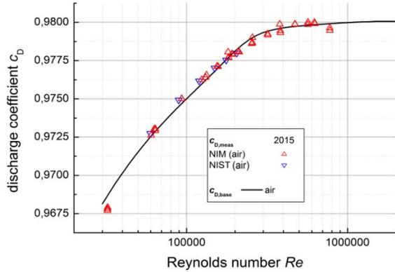
Figure 7: Data for nozzle NIST 2.5 mm.
