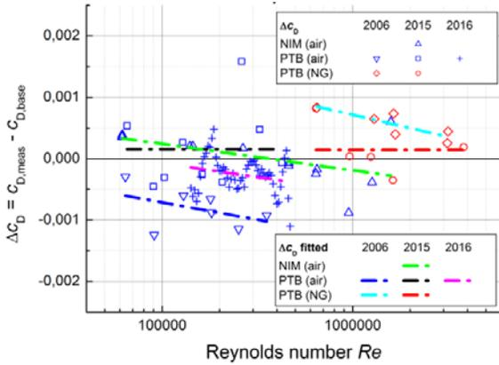
**Figure 2:** Differences  $\Delta c_D$  of single  $c_D$  values against the  $c_{D,base}$  function for the nozzle HD-9b. The  $\Delta c_D$  for each measurement series are approximated by a polynomial  $\Delta c_{D,fit}$ . Please refer to Figure 9 in the Appendix for plot of  $c_{D,meas}$  and  $c_{D,base}$ .
