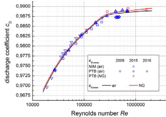
Figure 8: Data for nozzle HD-17b.
