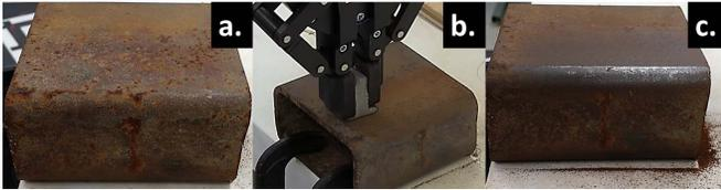
Fig. 14. Robotic cleaning of a rusty surface. (a) Before cleaning. (b) Ongoing cleaning pass. (c) After seven cleaning passes.
