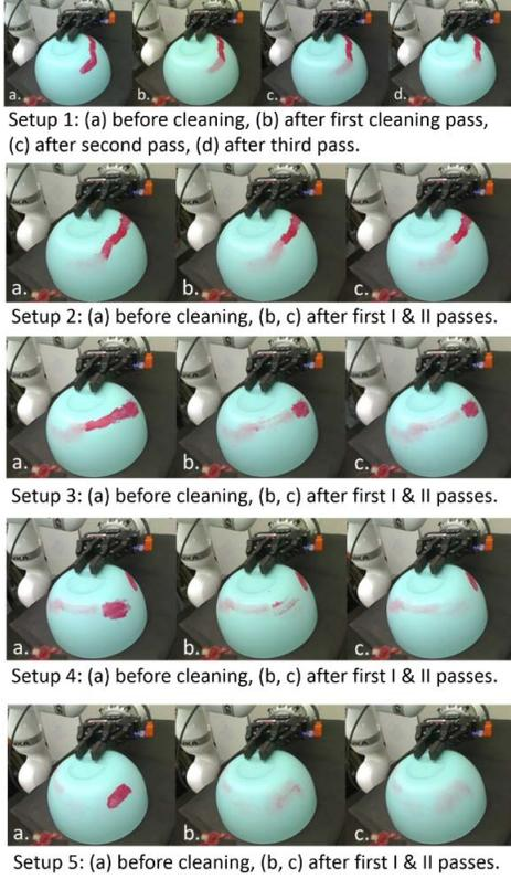
Fig. 11. Snapshots from a video showing execution of cleaning on the plastic bowl according to the setup plan comprising five setups. The part's surface is mostly convex.
