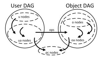
Figure 1: Diagram showing allowed edge relationships between the five different sets of NGAC node types.
