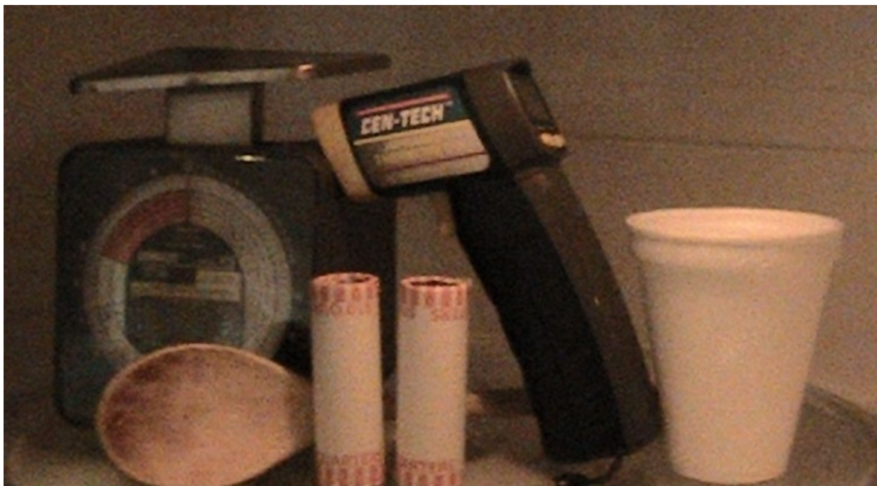
FIG. 1. The equipment used in this experiment is shown in the microwave oven with the glass plate visible. From left to right, the objects shown are the scale, the wooden spoon, the quarters, the IR thermometer, and a styrofoam cup.
