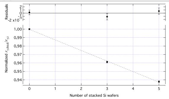
**Figure 15.** A plot of the ratio  $\frac{r_{\gamma,\text{thick}}}{r_{\gamma,\text{thick}}}$  versus number of silicon wafers stacked behind the <sup>10</sup>B target. A typical wafer is about 0.4 mm thick. The dashed line is a linear fit to the data; the residuals are shown in the upper plot. The error bars represent statistical uncertainty only.
