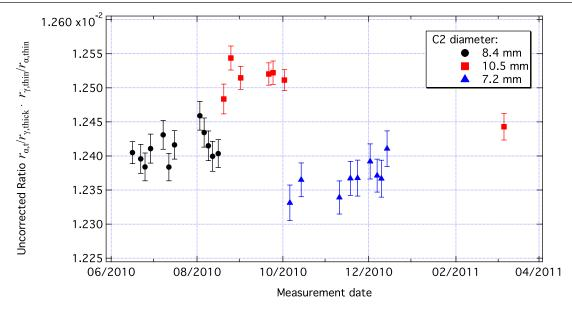
Figure 9. Plot of the results of the analysis for the three sizes of the C2 aperture. The error bars represent statistical uncertainty only.
