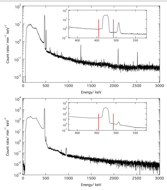
**Figure 8.** Top: plot of the gamma-ray spectrum from the thin <sup>10</sup>B target. The inset shows the region expanded around the 478 keV line, and the red lines indicate the analysis region. Bottom: plot of the gamma-ray spectrum from the thick <sup>10</sup>B target. The inset shows the region expanded around the 478 keV line, and the red lines indicate a typical analysis region.
