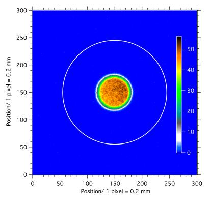
**Figure 20.** Beam images were acquired at the flux monitor deposit location with C1 = 15 mm and C2 = 7.2, 8.38, and 10.5 mm. The image for the largest collimation of C2 = 10.5 mm is shown here. The white circle corresponds to the edge of the active area of the <sup>6</sup>Li deposit.
