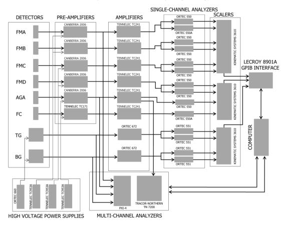
**Figure 6.** Electronics diagram for the alpha–gamma device and neutron monitor. FMA—FMD are the four neutron monitor silicon detectors, AGA is the alpha–gamma silicon detector, FC is an upstream fission chamber and TG and BG are the top and bottom HPGe detectors.
