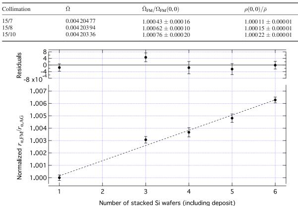
**Figure 21.** Measured ratio  $\frac{r_{\alpha,\text{FM}}}{r_{\alpha,\text{AG}}}$  as a function of the number of Si wafers stacked behind the monitor deposit. The dashed line is a linear fit, and the residuals are shown in the upper plot. The error bars represent statistical uncertainty only.
