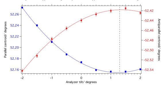
**Figure 12.** A tilt curve pair from the wavelength measuring apparatus. The solid lines are weighted fits to a parabola. The dashed line represents the tilt that best minimizes the parallel centroid and maximizes the antiparallel centroid. The error bars represent statistical uncertainty of the fit of the centroids.
