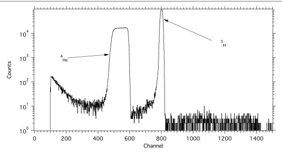
Figure 2. Typical pulse-height spectrum from <sup>6</sup>Li reaction products incident on a silicon detector in the neutron monitor.
