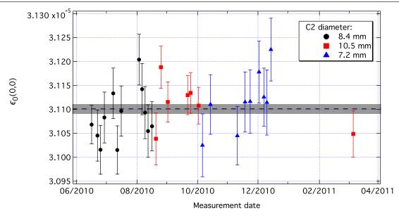
**Figure 22.**  $\epsilon_0(0,0)$  measurements for each of the three collimations. The dashed line is the weighted average of the values, and the gray band represents the  $\pm 1$ - $\sigma$  region. The error bars represent statistical uncertainty only.
