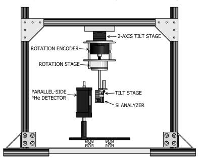
Figure 10. An illustration of the wavelength measuring apparatus installed on NG-6m.
