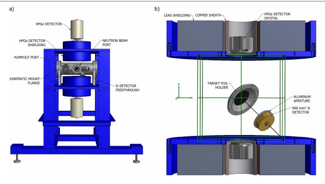
**Figure 1.** Illustrations of (a) the alpha–gamma device vacuum system (gray) in its support frame (blue) and (b) a section view of the alpha–gamma device showing the detection geometry; the neutron beam is incident on the target at the position of the green cross.
