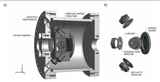
Figure 3. Illustrations of (a) a section view of the neutron monitor vacuum chamber and (b) a representation of the detection geometry.
