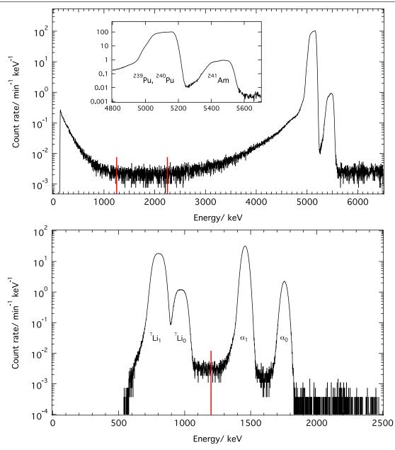
**Figure 7.** Top: charged particle spectrum from the  $^{239}$ Pu source. The inset indicates other isotopes that contribute to the alpha rate. The red lines indicate a typical region used for background subtraction. Bottom: charged particle spectrum from the thin  $^{10}$ B target. The red line indicates the position of a typical analysis threshold for counting the alpha particles.
