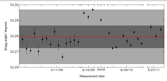
**Figure 13.** Plot of the measured  $\theta_{\text{Bragg}}$  angle. The centroid of the data (solid red line) is determined from a weighted constant fit ( $\chi^2/\text{d.o.f.} = 23.2$ ), and the dark shaded band corresponds to the  $\pm 1$ - $\sigma$  uncertainty of that fit. The uncertainty used for the wavelength determination was conservatively chosen to include the entire data set and is denoted by the light shaded band.
