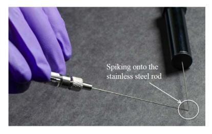
Figure 2. Illustration of direct loading of calibration liquid onto SPME stainless steel rod
