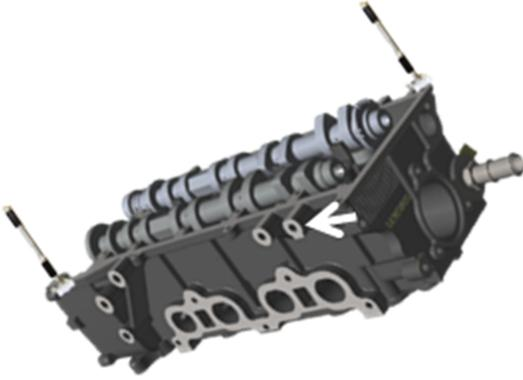
**FIGURE 7:** Two vector bars mounted rigidly to a part form a local frame which is tracked by a pose measuring system. The location of any POI on a part (marked by an arrow) can be determined from dynamically tracked pose and fixed location of the POI in a local frame. Uncertainty in pose measurement must be propagated to the POI.
