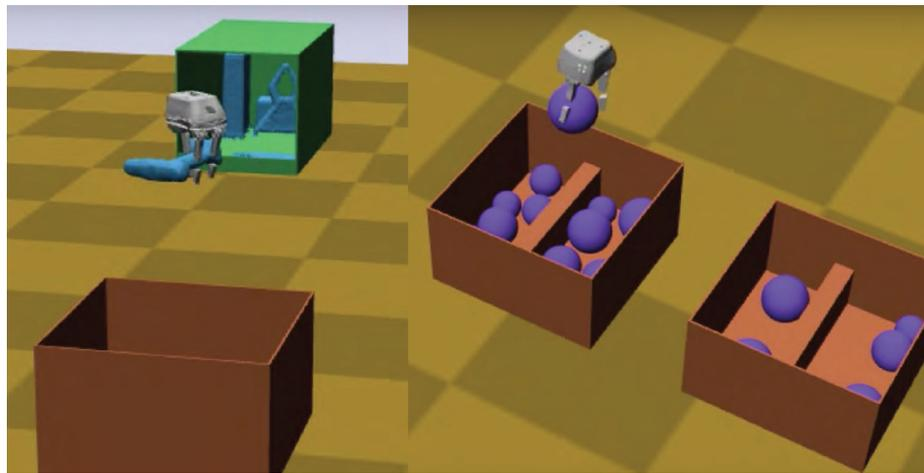
**Fig. 4.** Simulation task showing the extraction of as many objects as possible from a cluttered shelf and subsequent placement in a bin (left) and pick and placement of as many balls as possible from one bin to another (right).
