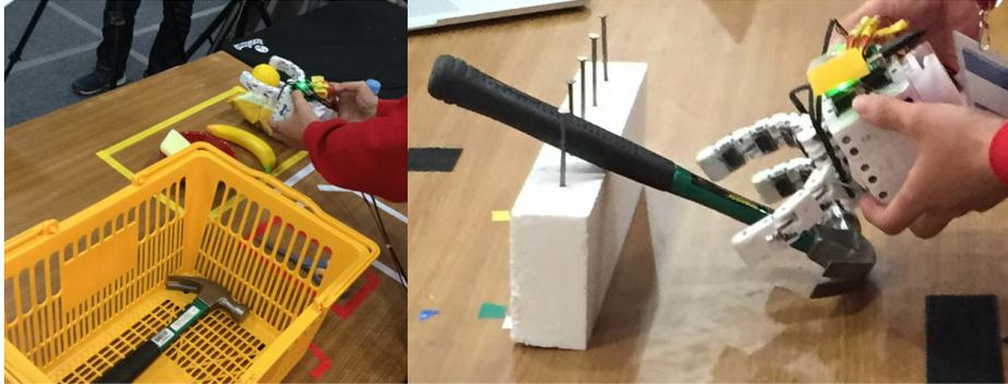
**Fig. 3.** Competitor hand design being used during the hand-in-hand track: pick and place (left) and hammer a nail task (right).
