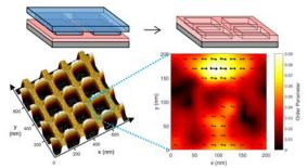
Mechanical deformation can be detected at the nanoscale by determining fluorophore orientation in single-molecule super-resolution optical microscopy.
