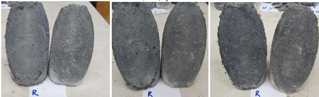
Figure 4. Photographs of representative dry and wet specimens after slant shear testing at 28 d for RM A. In each case, the RM half specimen is on the left side of the photo. The white patches (mostly in the top images) indicate where one material has adhered to the other surface.
