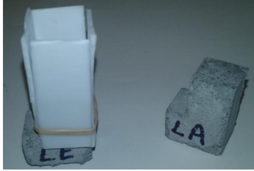
Figure 2. Photograph of typical L-shaped specimens with surrounding PTFE form (left) and with cut top surface (right) used for the radiography experiments conducted at the NIST Center for Neutron Research.
