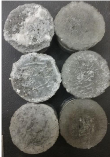
Figure 3. Photo of wet (left) and dry (right) pull-off test specimens for tests performed at NIST based on the newly proposed ASTM standard test method. The glossy white material is concrete that has adhered to the repair material specimen.
