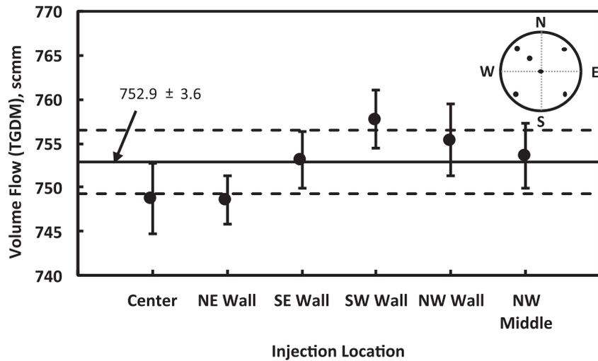
Fig. 7. Confirmation of uniform mixing of the tracer with single point injection at various locations at the exhaust duct inlet. Each point is the mean of 10 or more measurements, and the SDOM is represented by the error bars.
