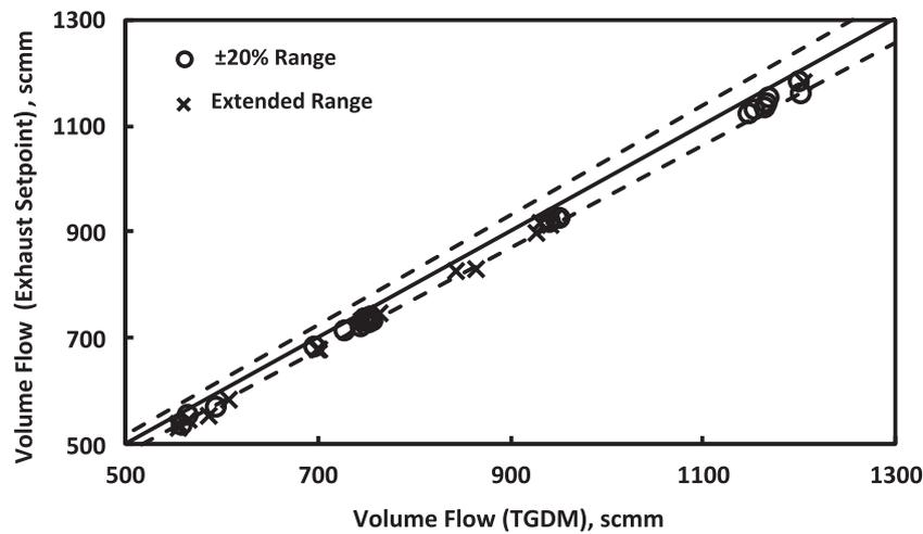
Fig. 9. Comparison of exhaust duct set-point flow (averaging pitot tubes) and exhaust flow determined using the TGDM. The solid line represents one-to-one agreement, while the dashed lines represent estimated limits of expanded uncertainty for the TGDM,  $\pm 3.5\%$ .
