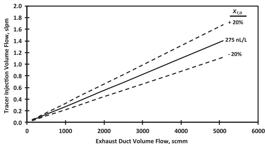
Fig. 4. Estimates of tracer injection volume flow required to generate optimal tracer volume fractions downstream.
