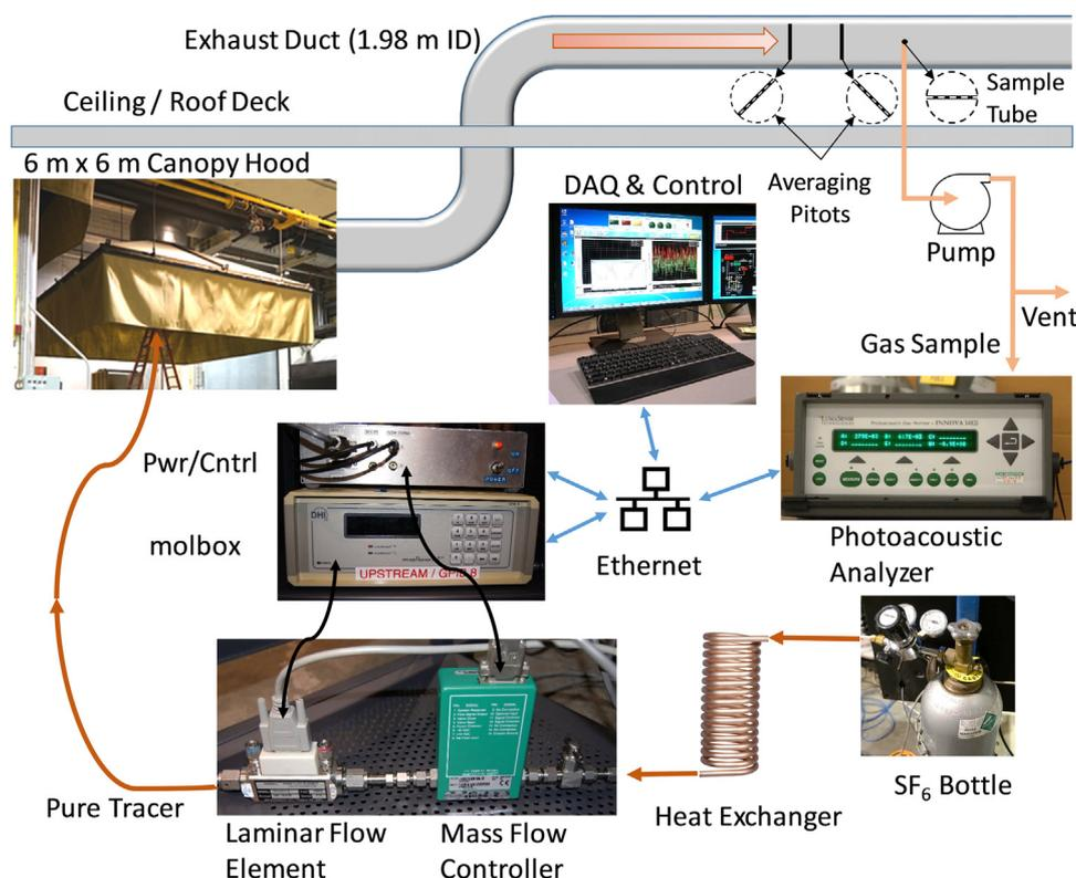
Fig. 2. Schematic of the experimental setup of the volume flow measurement in the 1.98 m ID exhaust duct using the tracer gas dilution method, constant-injection technique.
