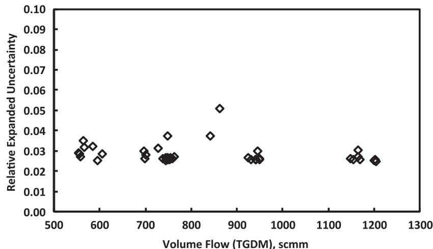
Fig. 8. Estimated uncertainty for the exhaust duct volume flow measurement using the TGDM.
