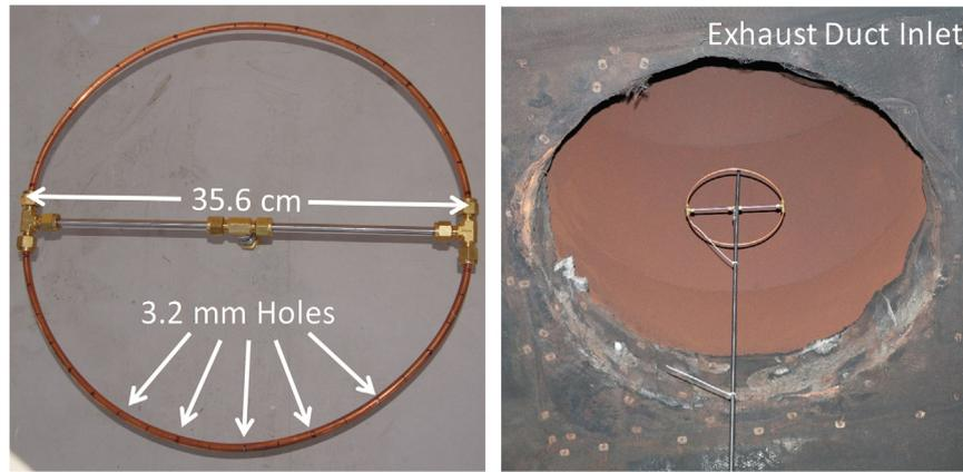
Fig. 3. Tracer injection ring (left photo); and tracer injection ring mounted inside the canopy hood at the inlet of the exhaust duct (right photo).
