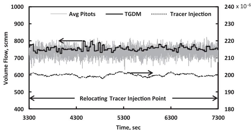
Fig. 6. Time trace for steady conditions of exhaust flow and tracer injection flow demonstrate a steady exhaust flow measurement by the TGDM during relocation of the tracer injection point at the inlet plane.
