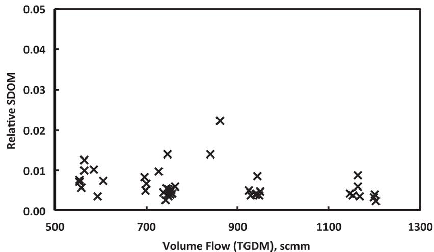
Fig. 5. Repeatability of the reported mean volume flow measurements.
