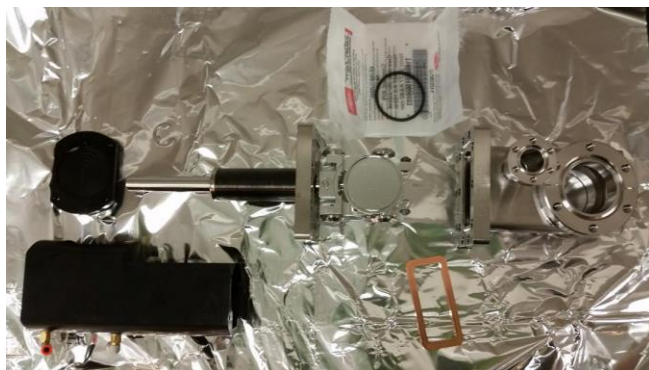
FIG. A1. (Color Online) Disassembled gate valve.
