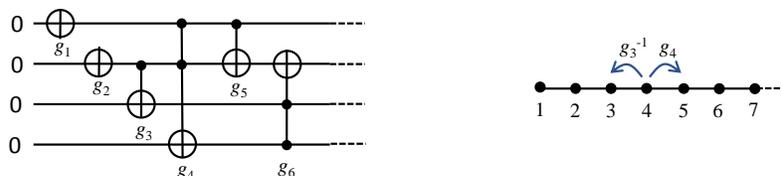
**Fig. 1.** A Brownian computation is described by a logically reversible circuit, whose gates are to be applied in some specified order. The dynamics of the Brownian computer are described by a random walk along a 1-dimensional chain.
