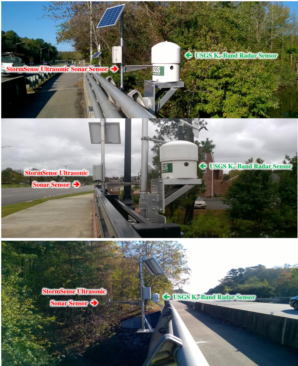
Fig. 5. Examples from three StormSense ultrasonic sonar sensors co-located in the field adjacent to USGS radar sensors in Virginia Beach for direct comparison of monitoring accuracy. These sensors will temporarily be stationed adjacent to each other for a period of 6-9 months to provide a long term data record for comparison of water level measurements, data transmission speeds, and solar power efficiency.
