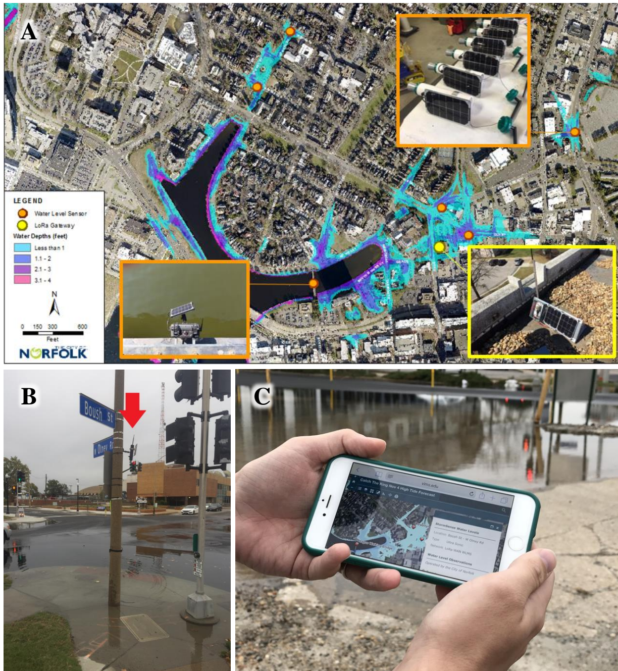
Fig. 4. A) Map of Norfolk's LoRaWAN ultrasonic sensor network established in The Hague. The group currently consists of one tide monitoring sensor mounted over The Hague Walking Bridge near where the USGS mounts their temporary rapid deployment gauge , and five inundation sensors, strategically positioned over frequently flooded streets. One such street is featured in B) at the intersection of Boush St. and Olney Rd. during the King Tide flooding on the morning of Nov. 4, 2017. C) The sensor data are currently publicly reporting water level observations in Tidewatch and the user interface provided by the manufacturer, Green Stream, Inc. ( https://greenstream.io/Dashboard ).
