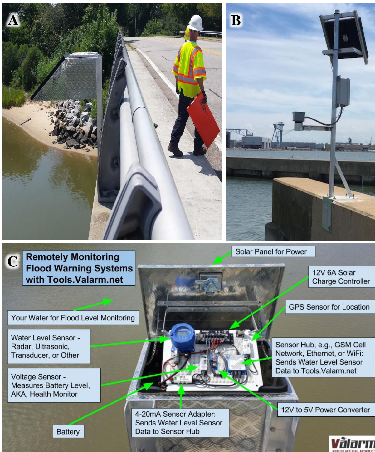
Fig. 3. Internal look at Newport News' sensor from Valarm: A) a standard bridge-mounted remote radar sensor control box configuration on the 16th St. Bridge over Salters Creek vs. B) a pole-mounted ultrasonic sonar sensor on a solid breakwater at Leeward Municipal Marina. C) The internal view of the control board and the sensor in panel A.
