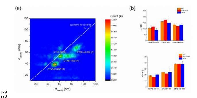
Figure 5 (a) Comparison of volume-based  $d_{vol}$  and mobility diameter  $d_m$  for a mixture of GNRs and gold nano-spheres. The heat bar represents the particle counts. (b)  $L_r$ ,  $d_r$  obtained from the mixture, individual GNRs and the TEM benchmark data.
