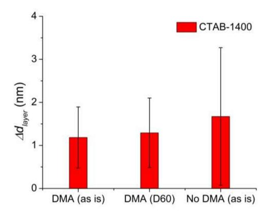
Figure S3. Measurement of adlayer thickness showing the effect of dilution and collection method. D60 indicates 60× dilution compared with the native suspension. The adlayer thickness observed with DMA size selection is compared with that without DMA selection. Neither the effect of dilution nor DMA selection has an obvious effect on adlayer thickness. Roughly 10 GNRs and multiple locations along each GNR were measured to yield an average and one standard deviation.
