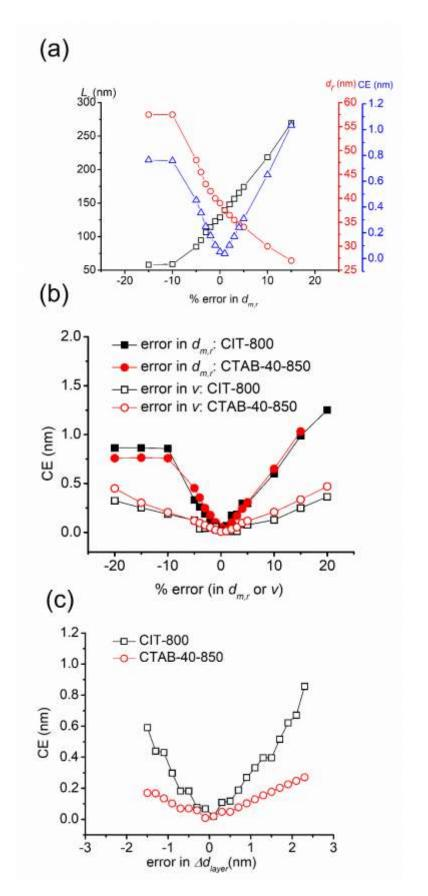
Figure 4. Robustness analysis of DMA-spICP-MS method. CE is defined as the combined error as defined in Eq. (5). (a) Change of  $L_r$ ,  $d_r$ , and CE with respect to perturbation in  $d_{m,r}$  measurement (CTAB-40-850 as an example). (b) Effect of both  $d_{m,r}$  and v perturbation on CE comparing two different dimensional configurations (CIT-800 vs. CTAB-40-850). (c) Effect of adlayer  $\Delta d_{layer}$  on CE comparing two different geometries (CIT-800 vs. CTAB-40-850).
