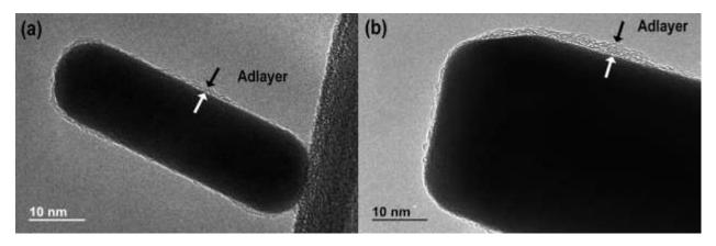
Figure 2. Two representative TEM images show evidence for a thin low density adlayer on the surface of GNRs. Both citrate and CTAB coatings were examined: (a) CIT-660 (b) CTAB-40-850
