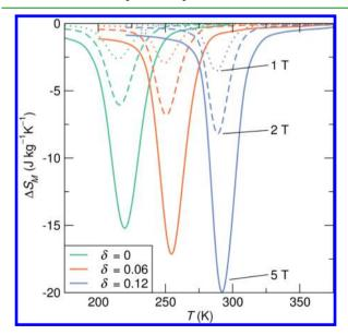
**Figure 8.**  $\Delta S_M$  for select fields of  $(Mn_{0.5}Fe_{0.5})_{2-\delta}P_{0.5}Si_{0.5}$  as obtained using eq 1 with temperature-dependent magnetization data collected at several fields.
