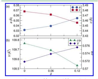
**Figure 3.** Unit cell parameters (a) *a* and *c* and (b) unit cell volume and c/a ratio for  $(Mn_{0.5}Fe_{0.5})_{2-\delta}P_{0.5}Si_{0.5}$  determined from Rietveld refinements of synchrotron powder diffraction data.
