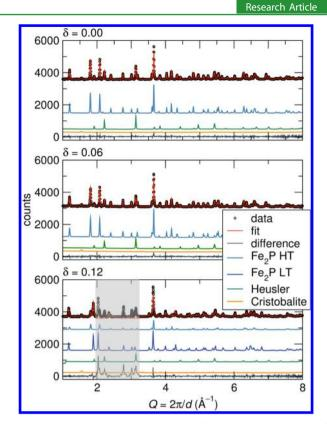
**Figure 2.** Neutron powder diffraction patterns of  $(Mn_{0.5}Fe_{0.5})_{2-\delta}P_{0.5}Si_{0.5}$  taken at 300 K and Rietveld fits to that data, showing individual contributions for the Heusler and cristobalite impurity phases. Peaks with significant magnetic contributions have been masked in  $\delta = 0.12$ .
