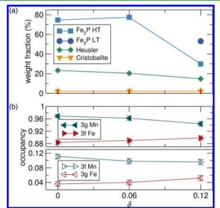
**Figure 4.** (a) Weight fractions of LT and HT  $(Mn,Fe)_2(P,Si)$ , and the  $(Mn,Fe)_3Si$  and cristobalite impurities, and (b) Mn/Fe site occupancies of  $(Mn_{0.5}Fe_{0.5})_{2-\delta}P_{0.5}Si_{0.5}$  as determined by joint synchrotron and neutron Rietveld refinements.
