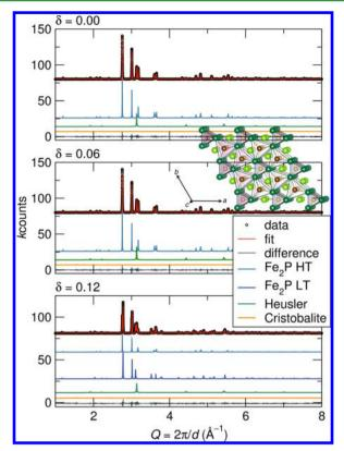
**Figure 1.** Synchrotron X-ray powder diffraction patterns of  $(Mn_{0.5}Fe_{0.5})_{2-.6}P_{0.5}Si_{0.5}$  taken at 300 K and Rietveld fits to that data, showing individual contributions for the impurity phases: Heusler  $(Mn,Fe)_3Si$  and cristobalite SiO<sub>2</sub>. The inset displays a view of the Fe<sub>2</sub>P structure of the materials discussed here, depicted as P-centered prisms formed by the transition metals.
