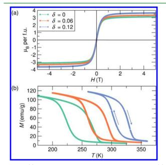
**Figure 7.** (a) Field-dependent magnetization taken at 100 K and (b) temperature-dependent magnetization data taken at H = 2 T of  $(Mn_{0.5}Fe_{0.5})_{2-8}P_{0.5}Si_{0.5}$ . The arrows indicate heating and cooling for the two branches of temperature-dependent data.
