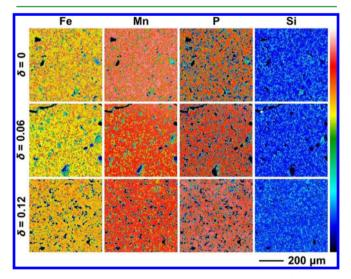
Figure 5. Electron microprobe X-ray backscatter maps of annealed pellets of  $(Mn_{0.5}Fe_{0.5})_{2-\delta}P_{0.5}Si_{0.5}$ . The color scale shows the relative weight percents of each element.
