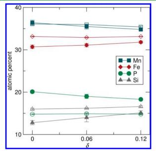
Figure 6. Elemental compositions of  $(Mn_{0.5}Fe_{0.5})_{2-\delta}P_{0.5}Si_{0.5}$  as determined from EMPA (filled markers) and XRF (empty markers).
