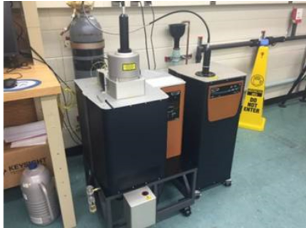
Fig. 3 DLF-1600 laser flash system
