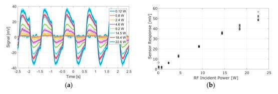
**Figure 3.** (a) Transient response of the miniature radiation pressure power meter to a microwave power. The slow creep of the sensor baseline is attributed to a high pass filter at the input of the oscilloscope (AC coupling). (b) Plot of the sensor's response peak signal against varying incident power; following the linear trend.
