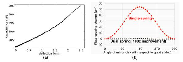
**Figure 2.** (a) Plot of the sensor's geometrical capacitance as a function of deflection. This is to determine the capacitance gradient, parasitic capacitance and initial plate spacing (comparison of two methods). (b) Plot of capacitor plate spacing as a function of the tilt angle. Zero angle corresponds to moveable mirror surface facing upwards and fixed plate downwards, 180° angle corresponds to fixed plate facing upwards and moveable electrode facing downwards.
