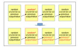
Fig. 2. Altering a pulse affects every future pulse in the hash chain
