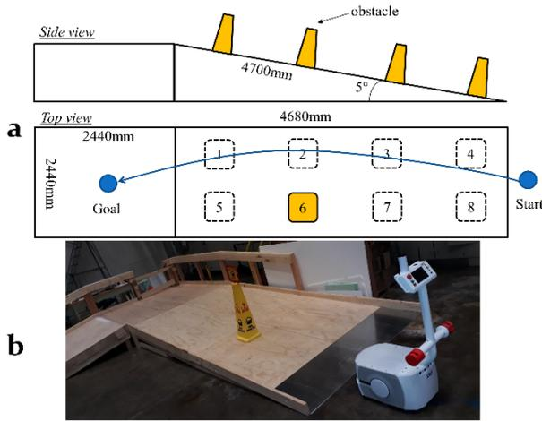
Fig. 10. (a) Drawings of eight different obstacles on a 5° ramp and (b) picture of an obstacle at location 6 on the ramp. The approximate A-UGV path avoiding the obstacle is shown from start to goal.
