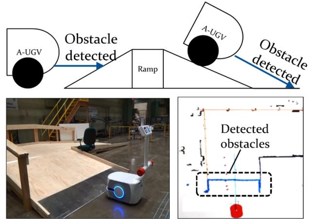
Fig 2. (top) Drawings of the ramp detected as an obstacle by the A-UGV. (bottom) Picture of the A-UGV in front of a ramp (left) and the ramp detected by the vehicle sensors (right).
