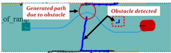
Fig. 11. Inefficient path generated due to obstacle (right) and ramp (left).
