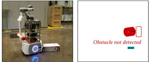
Fig. 9. A large, short box undetected by the A-UGV sensors.
