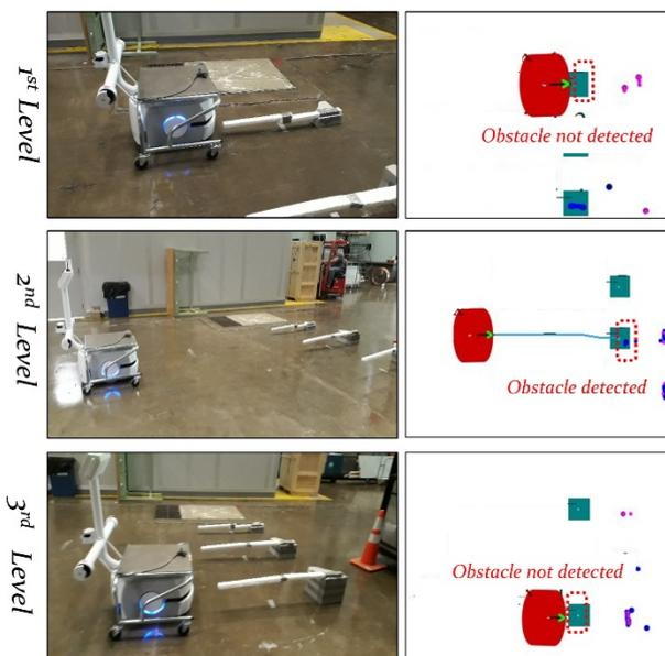
Fig. 8. Three overhanging obstacles with different heights being undetected (1<sup>st</sup> and 3<sup>rd</sup> level) and detected (2<sup>nd</sup> level) by the A-UGV sensors.
