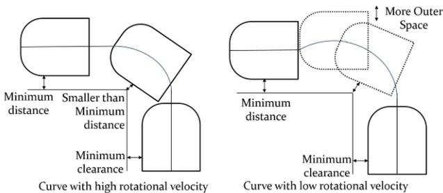
Fig. 1. Curved vehicle paths at high (left) and low (right) velocities.
