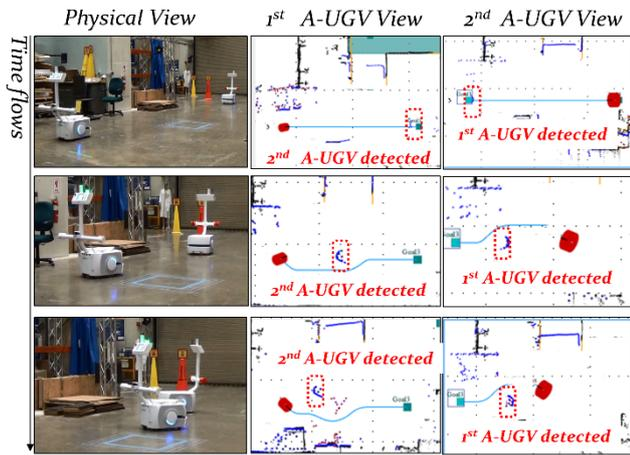
Fig. 7. Two vehicles approaching one another and recognized as obstacles by each other.
