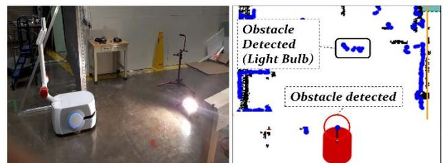
Fig. 6. Bright light detected as a (false) obstacle by the A-UGV obstacle detection sensors.
