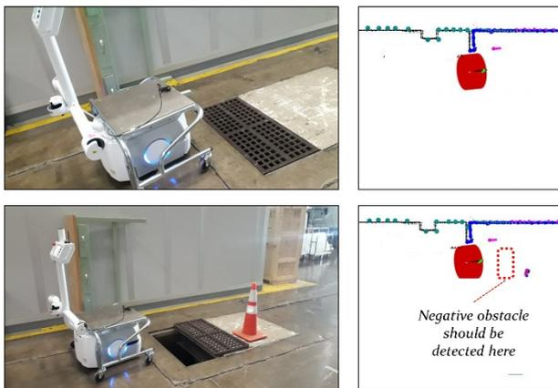
Fig. 5. A-UGV attempting to navigate across a covered (top) and uncovered (bottom) man-hole. The bottom image shows a negative obstacle not being detected by stock A-UGV sensors.
