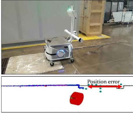
Fig. 3. A-UGV stuck on a raised surface resulting in vehicle position error. an example of a position error from the A-UGV being stuck on a threshold.
