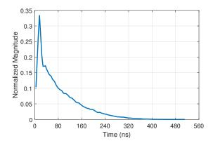
Fig. 6. The average CIR of all the measured CIRs at the steam plant.
