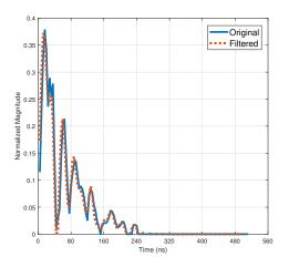
Fig. 2. Example showing the effect of data filtering on CIR.
