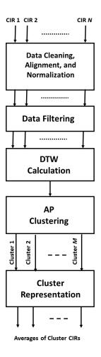
Fig. 1. Algorithm Block Diagram.
