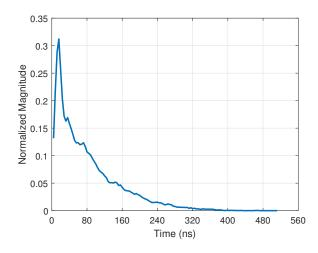
Fig. 3. The average CIR of all the measured CIRs at the Automotive factory.
