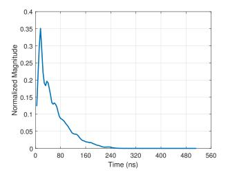
Fig. 9. The average CIR of all the measured CIRs at the machine shop.
