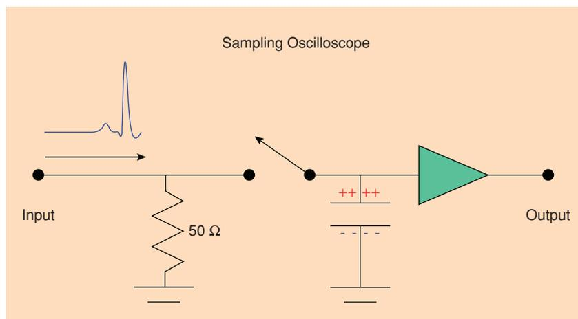
**Figure 1.** The operation of a sampling oscilloscope.
