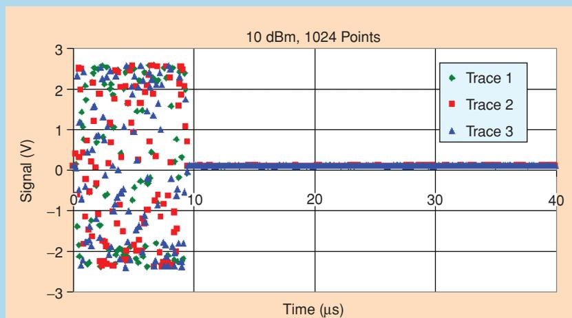
**Figure 11.** Measuring the RF power envelope through use of a sampling oscilloscope.
