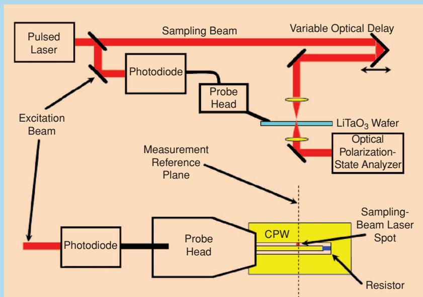
Figure 3. Sketch of NIST's electro-optic sampling system.
