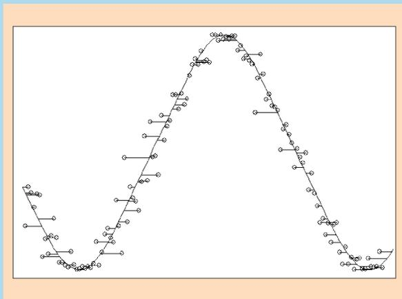
**Figure 6.** The circles show the sampled signal and the solid curve shows the estimated signal. The horizontal bars show the differences between the times estimated from the curve and the nominal oscilloscope timebase. (From [4].)
