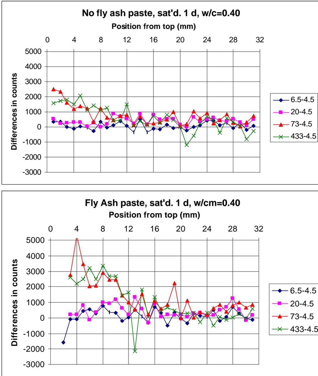
**Figure 6.** X-ray profiles (differences in counts) for pastes without and with fly ash, saturated for 1 d and then exposed to the chamber environment. All differences are relative to counts obtained for the 4.5 h specimens.
