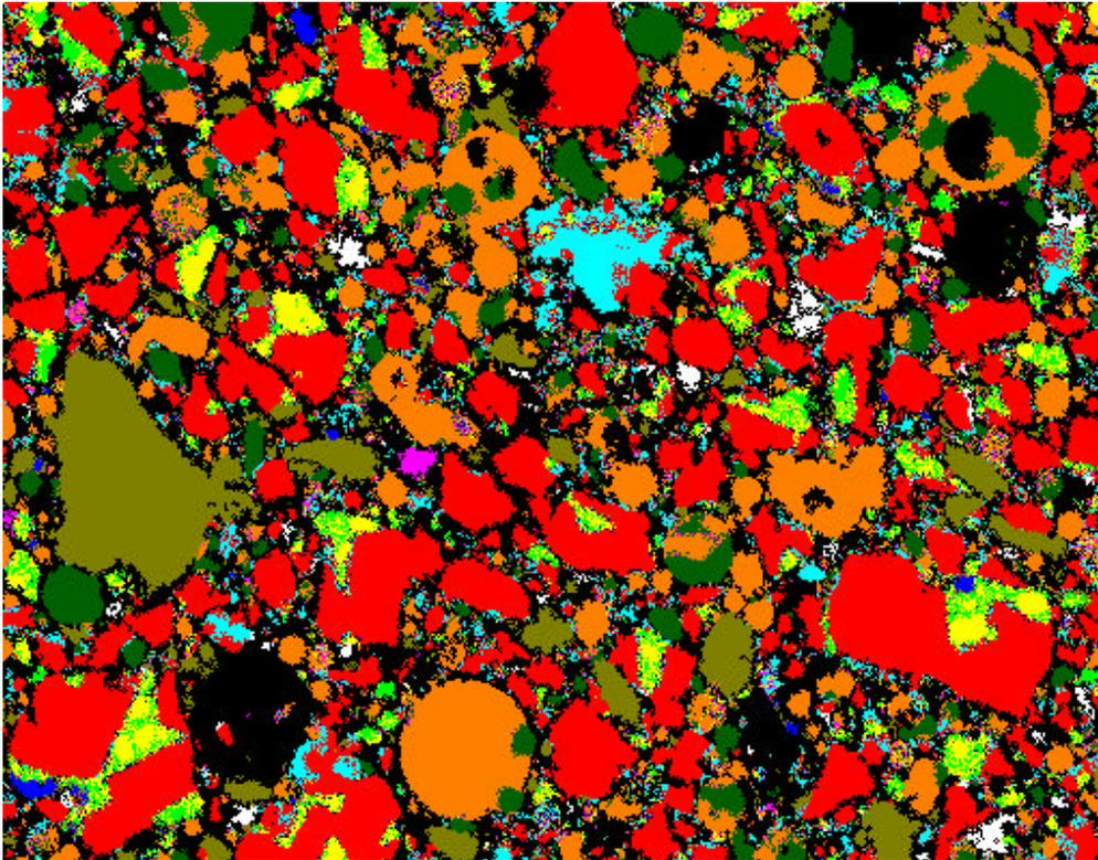
**Figure 2.** SEM/X-ray composite image of the blended cement containing about 20 % by mass fly ash. Colors are as in Figure 1, but additionally, orange is an aluminosilicate (fly ash), dark green is silica (fly ash), and dark blue is calcium aluminosilicate (fly ash).
