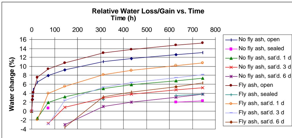
**Figure 3.** Relative water loss/gain vs. time for the cement pastes with and without fly ash exposed to various curing regimens. Positive values indicate a mass loss and negative values a mass gain (due to water imbibition).
