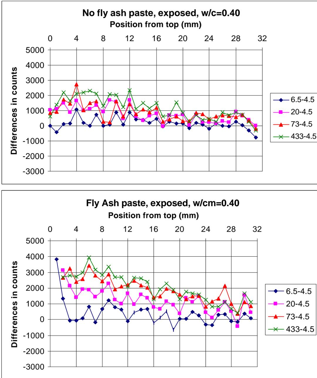
**Figure 4.** X-ray profiles (differences in counts) for pastes without and with fly ash, immediately exposed to the drying environment in the X-ray chamber. All differences (6.5 h, 20 h, 73 h, and 433 h) are relative to counts obtained for the 4.5 h specimens as indicated in the legend box. Positive values indicate a local water loss and negative values indicate a local water gain. The top (exposed surface) of the specimen is at position 0 and the bottom at position 32.
