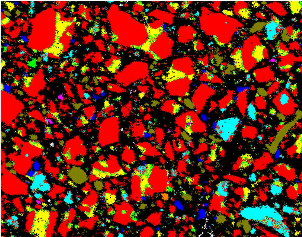
**Figure 1.** SEM/X-ray composite image of the ASTM Type I portland cement. Red is tricalcium silicate, aqua is dicalcium silicate, green is tricalcium aluminate, yellow is tetracalcium aluminoferrite, pale green is calcium sulfate, white is free lime, blue is potassium sulfate, and magenta is periclase. Image is 256  $\mu\text{m}$  x 200  $\mu\text{m}$ .
