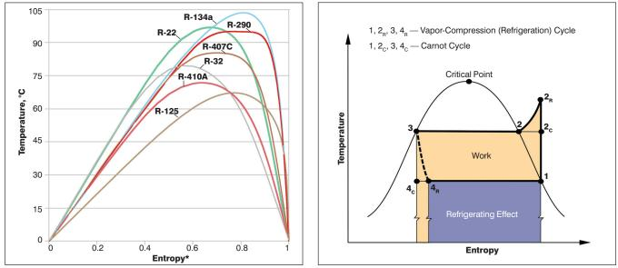
Figure 1 (left): Temperature-entropy diagram for R-22 and selected replacements (\*normalized entropy is plotted as a dimensionless ratio to facilitate comparisons). Figure 2 (right): Vapor-compression (refrigeration) cycle on temperature-entropy generalized diagram.
