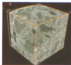
Fig. 5: Three-dimensional image (4.6 x 4.6 x 4.7 mm [0.181 x 0.181 x 0.185 in.]) of a portion of the microtomography data set for the IC mortar obtained immediately after mixing and casting
