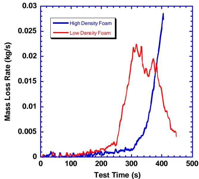
**Figure 10. The mass loss rate for a configuration 8 flaming fire test (bedroom, high density foam) and a configuration 5 flaming fire test (living room, low density foam).**
