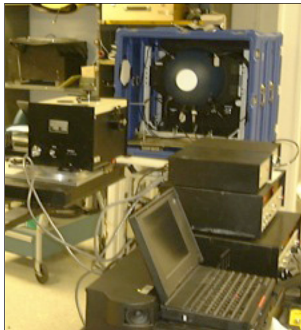
Figure 5. NPR: The NPR and the GSFC scanning monochromator during the EOS intercomparison at NASA's Ames facility in 1999 [18]. The NPR system is packaged in two shipping containers, the sphere is shock-mounted in the upper blue case, and the electronics in the lower white case.
