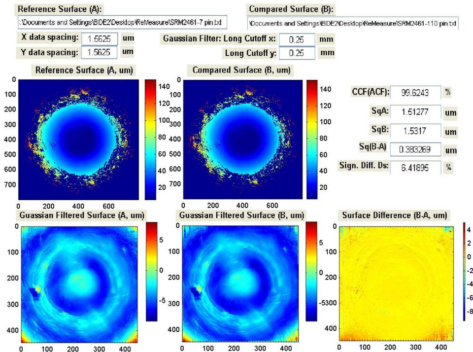
Figure 3. User screen showing the correlation of the firing pin impressions on two units of SRM 2461, the standard cartridge cases reproducibly fabricated by electroforming.
