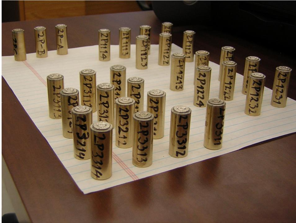
Figure 1. Typical batch of SRM cartridge cases. The buttons on top are the electroformed Ni replicas, which are bonded to turned cylindrical bases. The outer diameter is about 13 mm.
