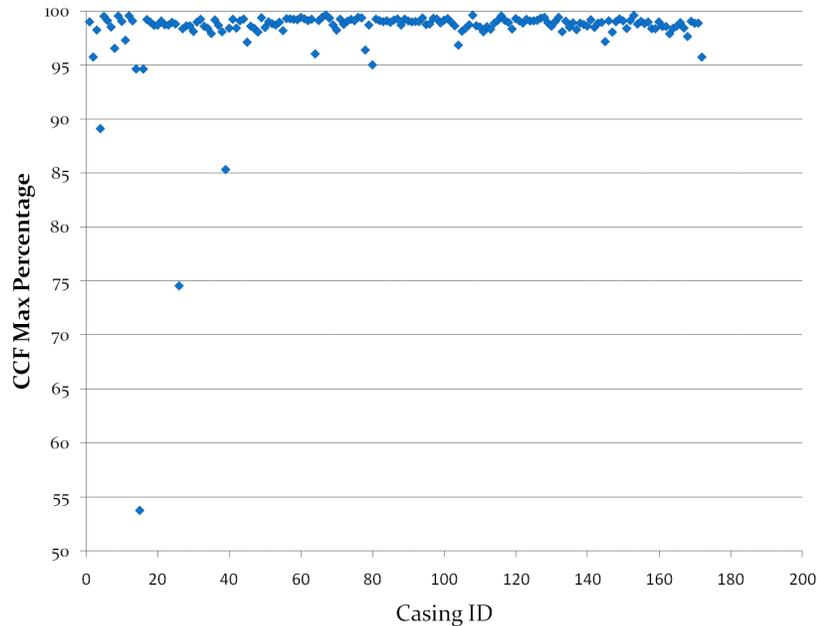
Figure 4. Cross-correlation maxima for the topographic images of firing pin impressions of 173 SRM cartridge cases, using SRM unit #007 as a master.
