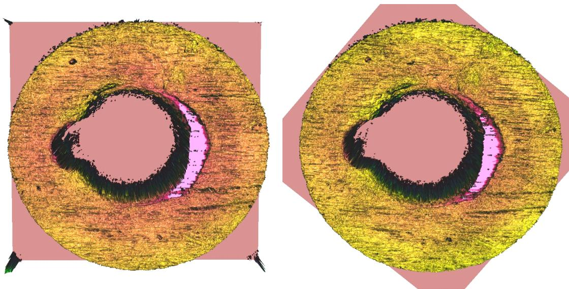
Figure 6. Topographic images of breech face impressions obtained with confocal microscopy using a 10× objective: (left) at 0° orientation and (right) at 35° orientation. The latter image has been rotated manually here to be close to the optimum orientation for correlation. The cross-correlation maximum between the images is 0.95.
