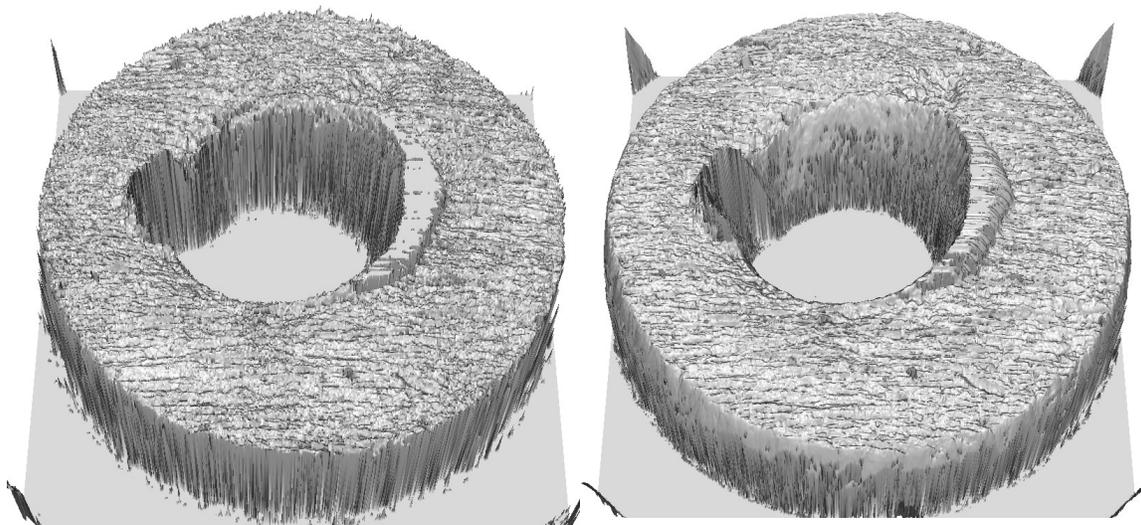
Figure 5. Topographic images of breech face impressions obtained with confocal microscopy using a 10× objective (left) and a 20× objective (right).
