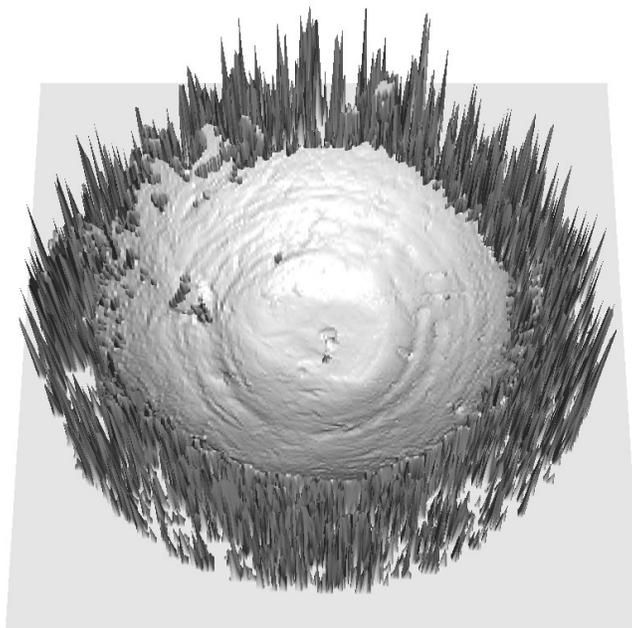
Figure 2. Topographic image of the firing pin impression on SRM 2461, Standard Cartridge Case, Unit #007. The outside border region contains numerous outliers and dropouts, so only the data in the center are used in the analysis.
