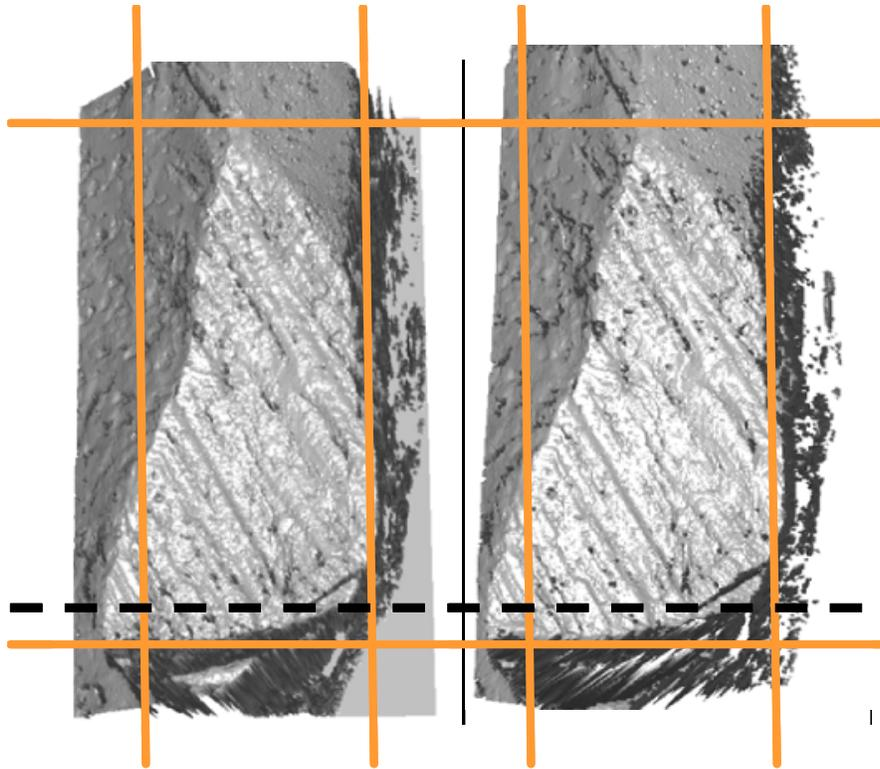
Figure 7. Comparison of ejector mark topography images from two different units of SRM 2461, #001 on the left and #011 on the right. The inner rectangles designate the approximate limits of the areas that were correlated after trimming by the Gaussian filter (solid line) then further trimming of unreliable data points (dashed line).
