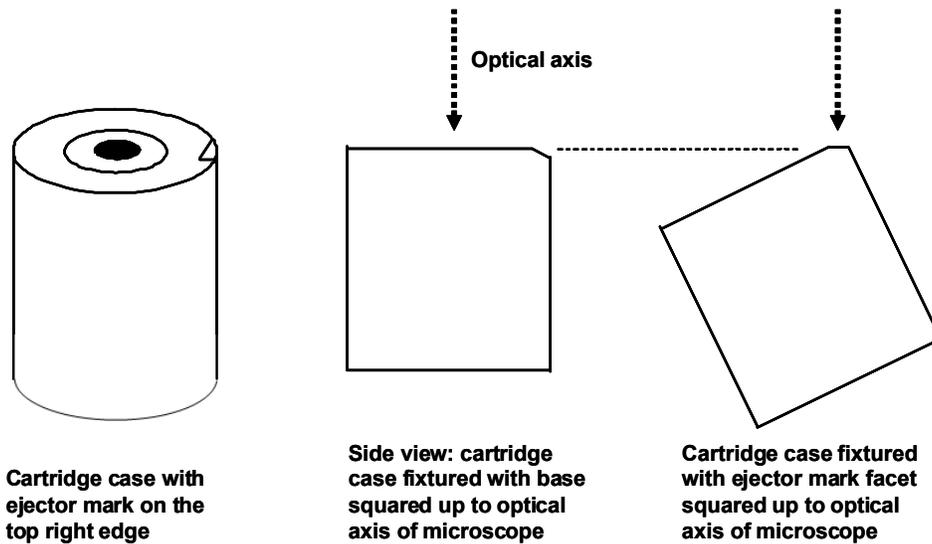
Figure 8. Two orientations for microscopic inspection of cartridge case ejector mark; (middle) customary setup, (right) setup used to optimize the signal-to-noise and minimize dropouts and outliers for measurement of surface topography with confocal microscopy.
