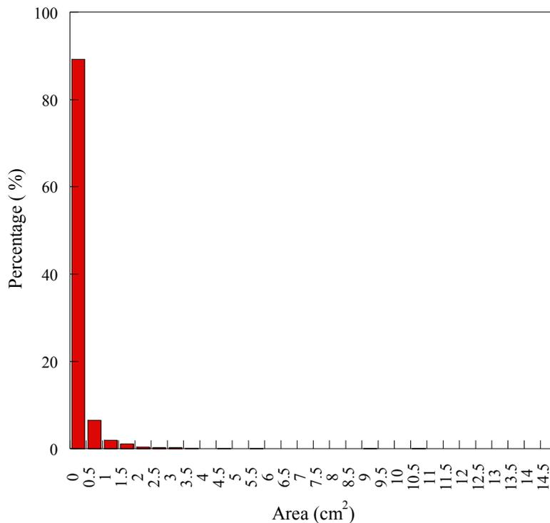
The size distribution of holes in the vertical trampoline safety net wall was observed to be similar to that of the trampoline base. However, the trampoline wall was constructed of a different material than the base which has not lent itself to effective digital image analysis of the burn patterns.
