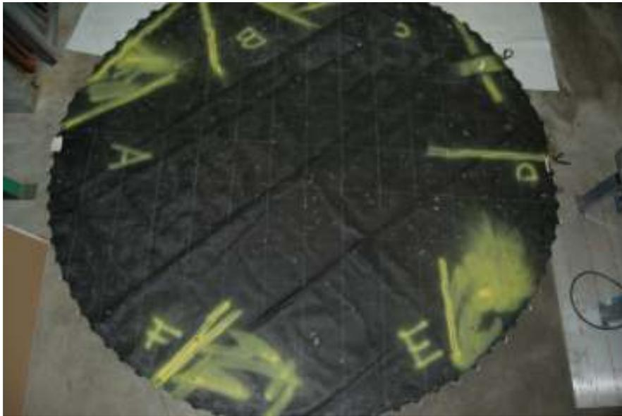
Figure 2 displays a digitized image of one of the quadrants of the trampoline. This image has been converted to an 8 bit grayscale image. Image analysis software was then used to determine the area of burn holes (see outline in image). The area of the burn pattern was subsequently calculated by converting the pixel area using an appropriate scale factor.
