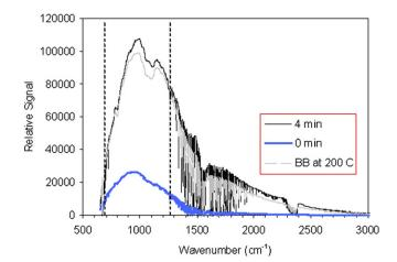
Fig. 3. The relative FTIR signal measured at two times during an experiment burning carpet, padding, and wood. For comparison, measurement of the relative signal of a blackbody source at 200 °C ( $\pm 5$  °C) is also shown.
