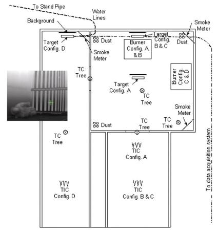
Fig. 2. Plan view of representative full-scale fire test layout with instrumentation and inset showing upper and lower thermal bar and mannequin targets.
