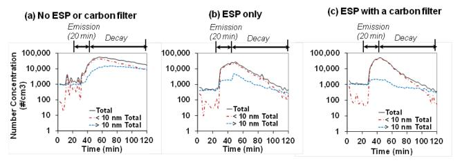
**Figure 3** Particle concentrations (a) neither ESP nor carbon filter operating (central fan off); with ESP only operating; (b) with ESP and an activate carbon media filter operating.
