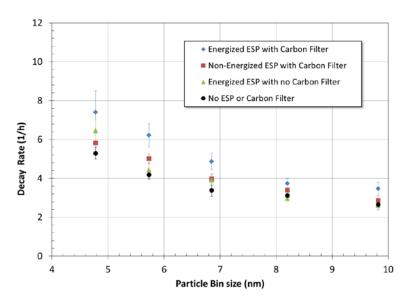
**Figure 4:** Comparison of particle decay rates for particle sizes less than 10 nm for experiments with ESP on and off. Central furnace fan was running continuously for all three cases. Error bars show the standard deviations of the averages.
