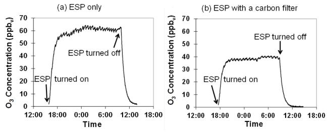
**Figure 2** Ozone concentration profile examples: (a) ESP only and (b) ESP with a carbon filter downstream – this carbon filter was one of three commercially purchased activated carbon filters, which was the most efficient filter in removing ozone among the filters tested.
