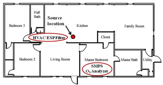
Figure 1. Test house layout with locations of the particle source, ESP and monitoring equipment
